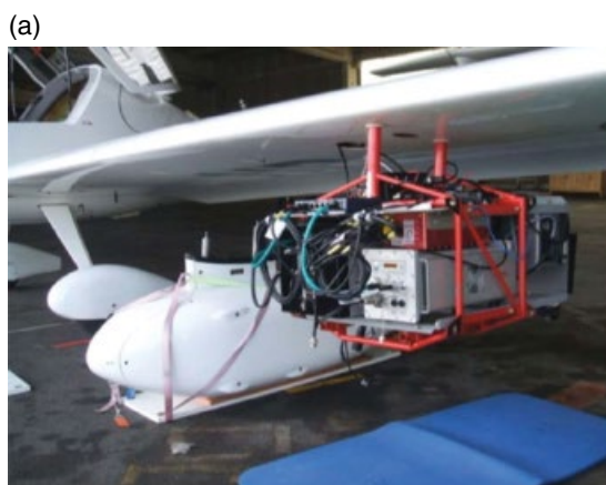
Figure 2.5 Examples of an airborne LiDAR system: an auxiliary pod fastened beneath the wing of a lightweight Dimona aircraft (a) and a terrestrial laser scanner
