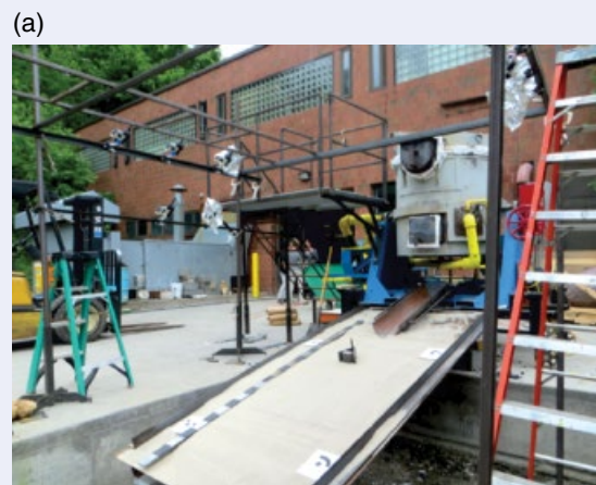
Figure B7.2ii Syracuse Lava Project experiments: experimental setup with five ISfM camera visible on the far side of the experiment platform (a); camera detail with wireless trigger and aluminium foil heat shield (b); natural colour point cloud of one of the experimental lava flows (c); and elevation coloured point cloud of the same flow (d).
