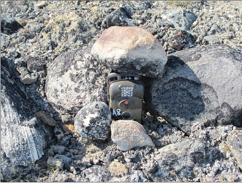
Figure 4.5 One time-lapse trail camera (out of an array of 15) deployed in West Greenland to derive
