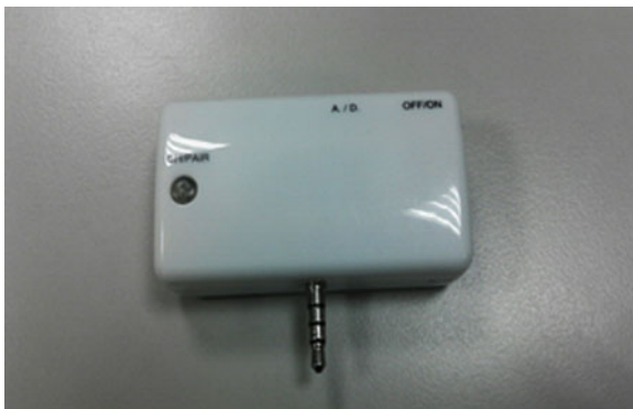
Fig. 4 The 2.4 GHz wireless audio transmitter
