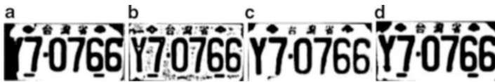
Fig. 12 (a) By Otsu. (b) By Niblack. (c) By MAT. (d) By proposed
