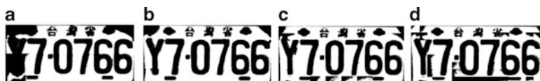
Fig. 11 Effect of different block sizes. (a) Binary image ( 4 \times 4 ). (b) Binary image ( 4 \times 8 ). (c) Binary image ( 8 \times 8 ). (d) Binary image ( 8 \times 16 )
