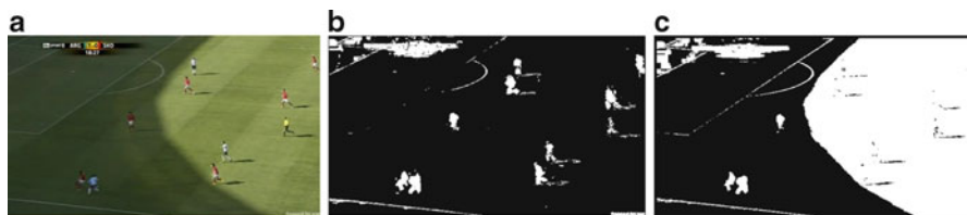
Fig. 6 Comparisons of playfield segmentation results between the proposed method and [2]. (a) Original image. (b) Our proposed method. (c) Results using ref. [2]
