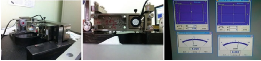
Fig. 4 The adjustment jig of PSD lens module and PSD displayed position on screen
