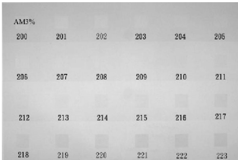
Fig. 4 The density calibration chart with 3 % AM halftone dots (in K) and varied grayscale values of FM halftone dots (in YMC)
