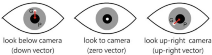
Fig. 4 Three glint–pupil difference vectors ( GPs )
