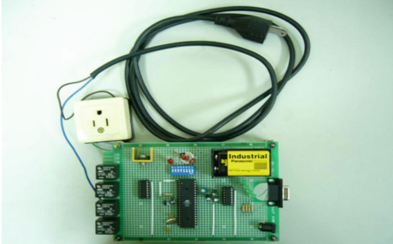
Fig. 4 An accomplished control circuit board used to switch the state of the household appliances when the coordinator sends a control code to RFD that actuates the 8951 microprocessor
