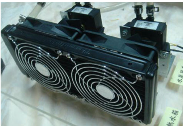
Fig. 5 The radiator and water pump
