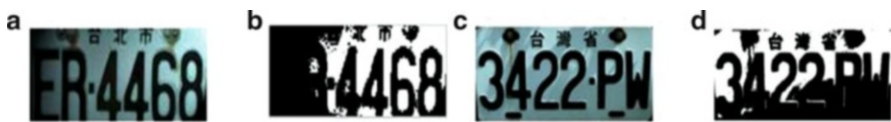
Fig. 9 Nonuniform illuminated LP and their Otsu binary images. (a) Nonuniform illumination. (b) Binary by Otsu. (c) Nonuniform illumination. (d) Binary by Otsu
