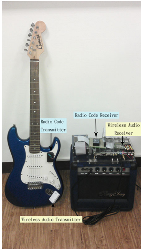
Fig. 12 The wireless electric guitar with digitally integrated effector
