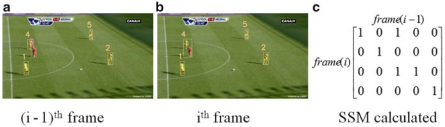
Fig. 5 SSM of two frames. First row shows players in merge state and second row with players in split state. Third row in disappearing state and forth row shows the normal case
