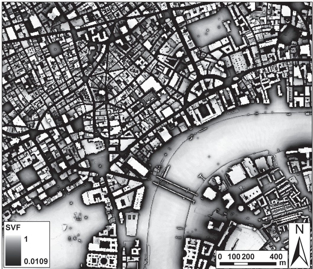
FIGURE A.3 Sky view factor (SVF) and location of a UK Met Office climate station (SJP, St James's Park) in central London. SJP can be seen to have a much higher SVF than the surrounding urban area. Annotated figure from Lindberg and Grimmond (2010).
