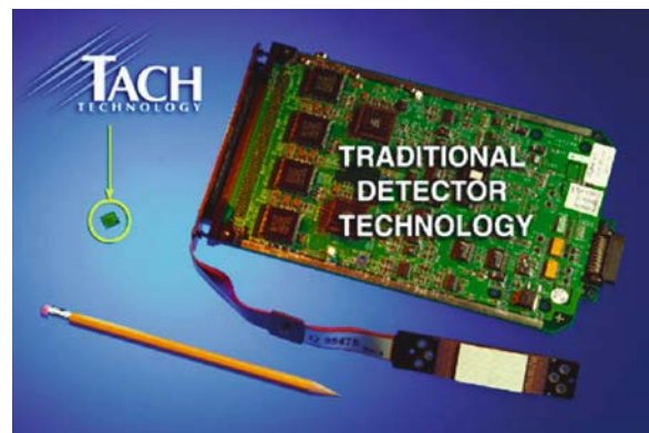
Fig. 4.14. The spatial requirements of an increased number of detector rows and the exorbitantly increased data rate necessitated the development of data acquisition systems with tiny application-specific integrated circuits (ASICs) that replaced the traditional circuit boards (courtesy: Philips Medical Systems)
