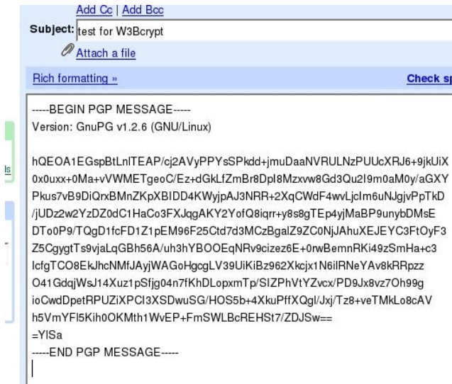
Fig. 1. Encrypted Data. After the text is selected and W3Bcrypt is invoked via the context menu, the selected text is replaced with ASCII-armored data. This data can be decrypted by the receiver either manually or automatically.
