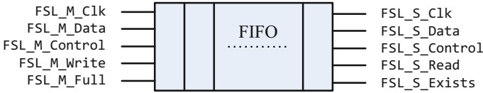
Fig. 4.14 FIFO-Based communication for the FSL bus
