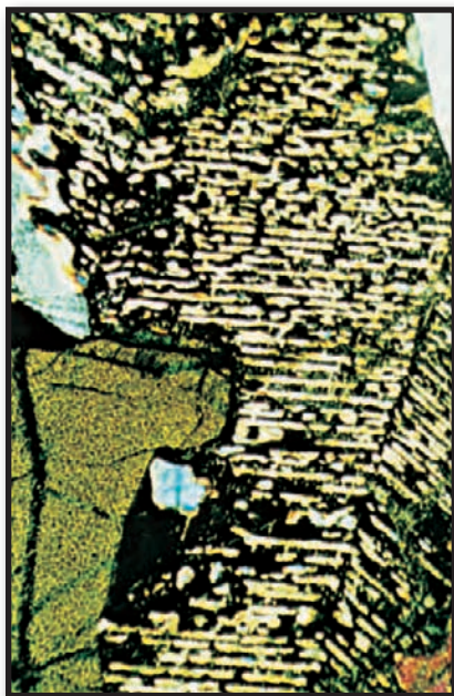
A micrograph of a twinned crystal of inverted pigeonite from a gabbro. Courtesy of G. Malcolm Brown
