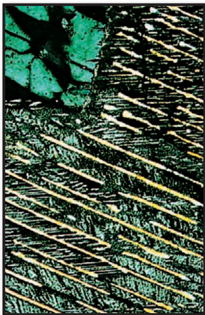
A micrograph showing a sample of inverted pigeonite from a slowly cooled gabbro. The augite lamellae here are relatively wide, separated from the enstatite host (magnified about 70.4×). Courtesy of G. Malcolm Brown
