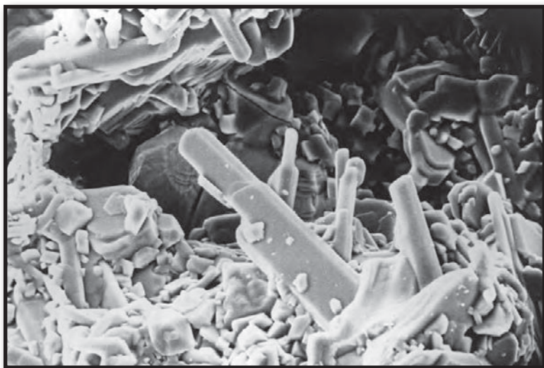
A scanning-electron-microscope photograph of pyroxene and plagioclase crystals (the long and the short crystals, respectively) that grew in a cavity in a fragment of Moon rock gathered during the Apollo 14 mission. NASA
