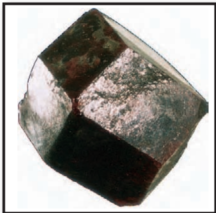
Dodecahedron, a common crystal form of garnet. Miller Museum of Geology and Mineralogy, Queen's University at Kingston, Ont., Can.
