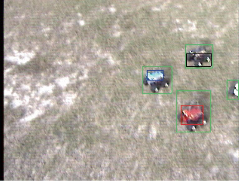
Fig. 6.26 Identification of a team where only three out of four UGVs are visible.
