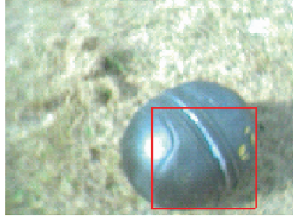
Fig. 6.16 Test image under different lighting conditions. A minimum bounding rectangle superimposed over the area that the algorithm detected the object.
