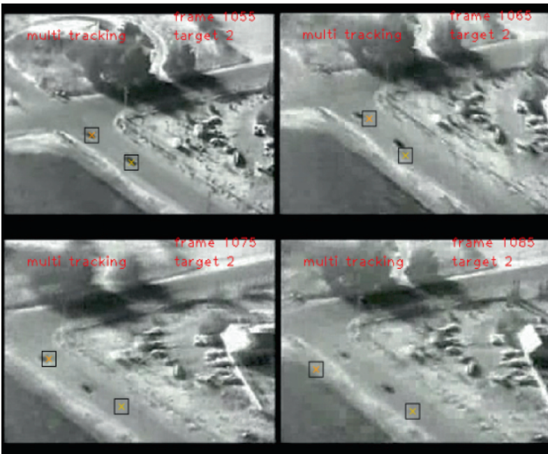
Fig. 6.40 Severely abrupt motion results in image blur and loss of track.
