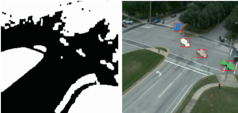
Fig. 6.31 Extraction of regions using connected components and a size filter. Notice the rejection of very large and very small blobs.
