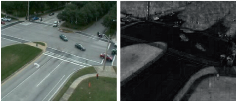
Fig. 6.28 The RGB input image in the left is converted to HSI. The saturation component is shown in the right.
