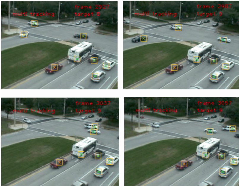
Fig. 6.36 Tracking is maintained despite the unpredictable motion of the VTOL and the parallax inducing motion of the vehicles.
