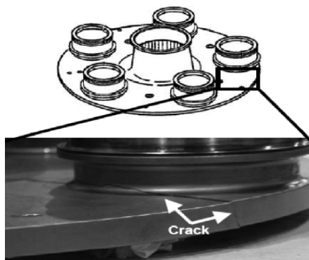
Fig. 3.1 The crack of planetary gear carrier plate of the UH-60A helicopter.
