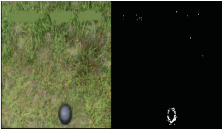
Fig. 6.13 Another input-output pair of images. Notice that some pixels on the top of the image have been misclassified as belonging to the object of interest.
