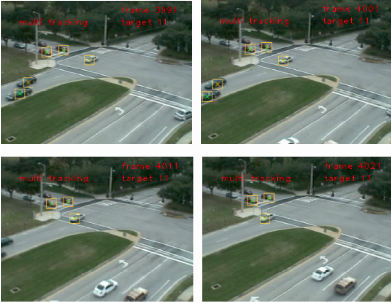
Fig. 6.35 Tracking is terminated when targets, such as the two vehicles at the right side of the frame, exit the field of view.
