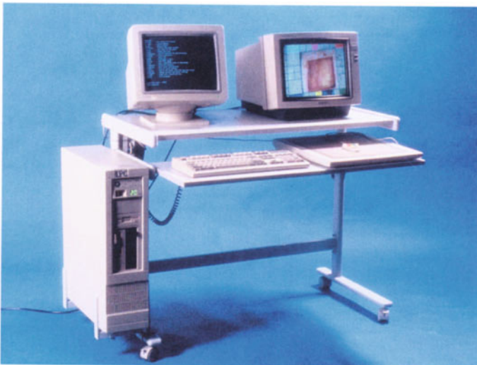
Fig. 4. The computer image analysis system: an IBM-compatible personal computer, a frame grabber, a VGA monitor and an RGB monitor, and a digitizing tablet
