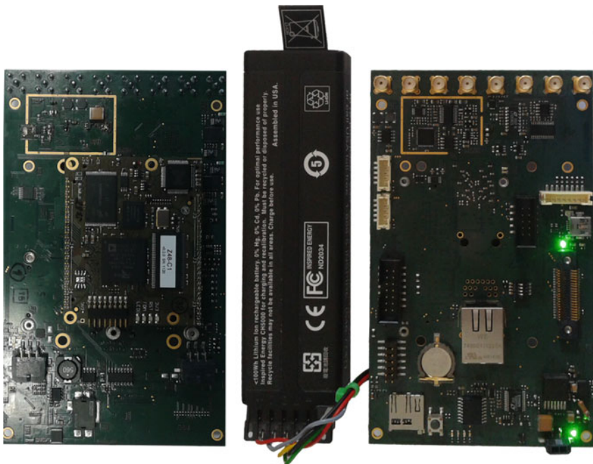
Fig. 2. UPER-MB powered by Inspired Energy Li-ION smart battery. Bottom view with Z48-C1 on the left and top view on the right
