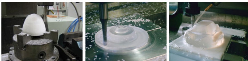
Fig. 1.11 Lens fabrication by CNC milling machine technique
