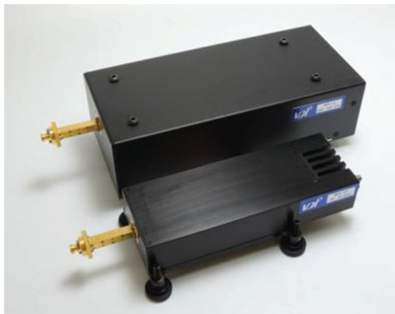
Fig. 12.5 A size comparison of the original modules (11" x 5" x 3") with the new mini-modules (8.5" x 3" x 1.5"). The volume is reduced by 75% and the weight by more than 50%
