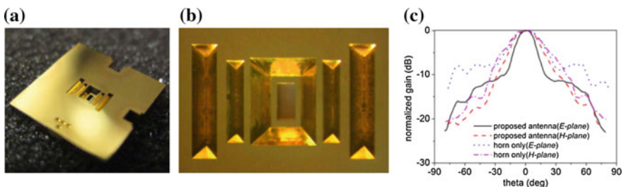
Fig. 4.10 a Micromachined V-grooves antenna. b Close view of manufactured antenna. c Normalized E- and H-plane for patterned antenna (black and blue dotted curves) and horn antenna (red and pink dashed curves). Reprinted with permission from John Wiley & Sons, Ltd
