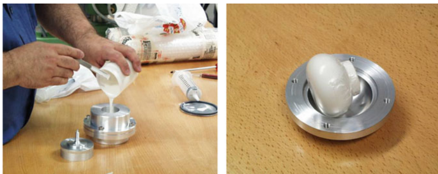
Fig. 1.12 Lens fabrication by molding technique
