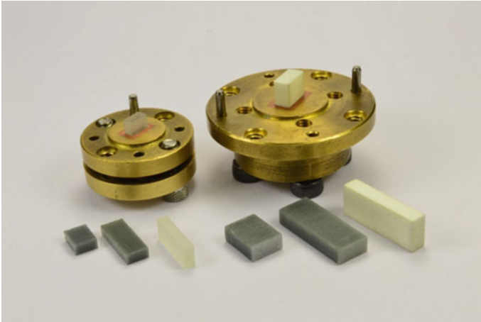
Fig. 1.9 Example of waveguide short-circuited sample holder for V-band and a few dielectric samples [51]
