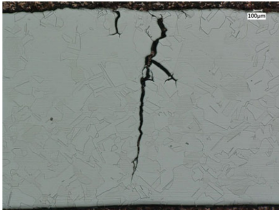
Fig. 22 Micrograph of the cross section prepared through the tube #17 through-wall crack tip. OD surface is along top edge. Electrolytic 10% oxalic etch
