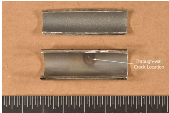
Fig. 12 Photograph taken after cutting the piece open clamshell-style to reveal the ID surface. The through-wall crack location is indicated
