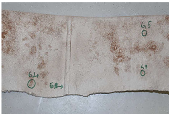
Fig. 2 Strip from elbow ND 500 × 6.3 mm, inner surface after sand blasting and wall thickness measurement, markings show measured minimum wall thickness values
