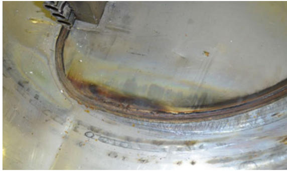
Fig. 7 Higher magnification view of the tight radius region showing the most pronounced heat tinting
