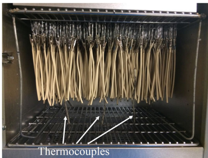
Fig. 3 Photo of oven chamber containing rack of XLPE specimens
