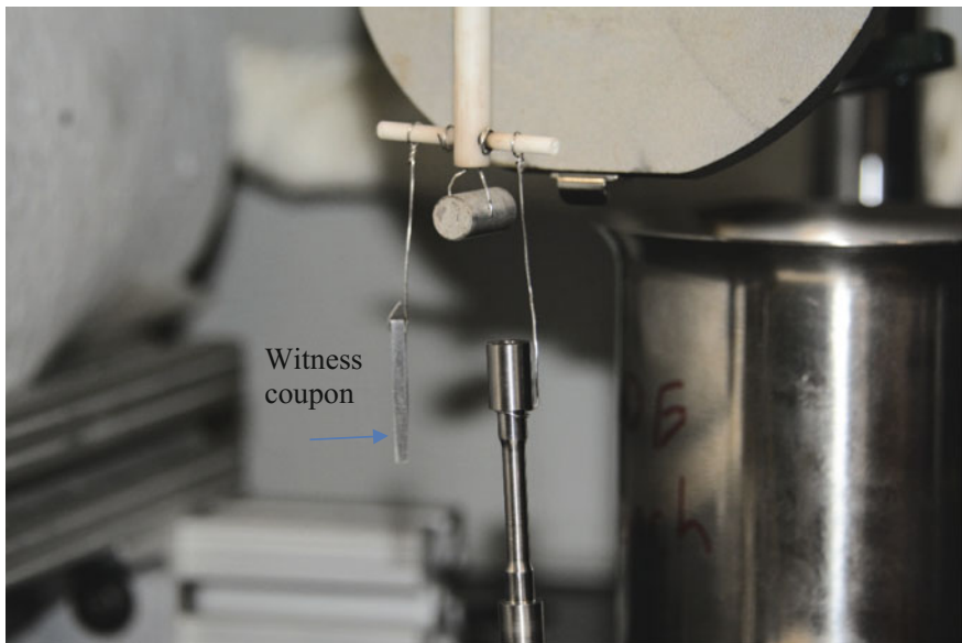
Fig. 3 Alumina specimen hanger with integrated thermocouple. The tensile specimen is exposed with a witness coupon
