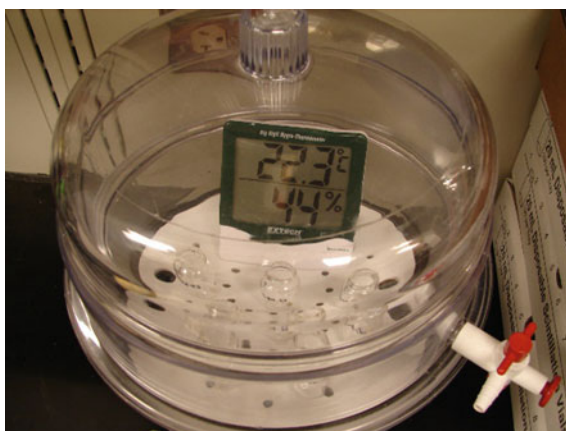
Fig. 1 Vessel used to pre-condition samples overnight at 44% humidity and room temperature
