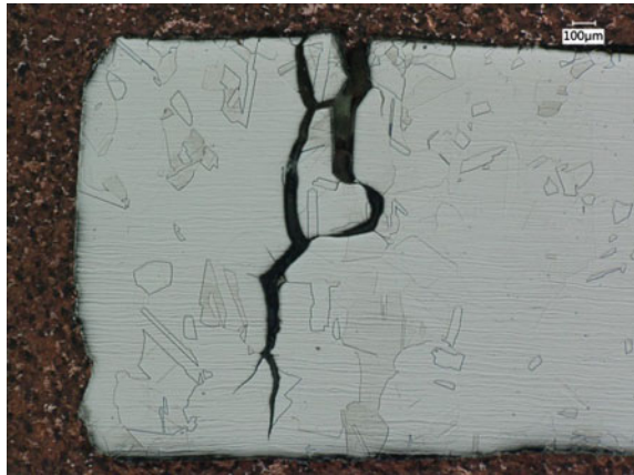
Fig. 24 Tube #17 secondary crack. Electrolytic 10% oxalic etch
