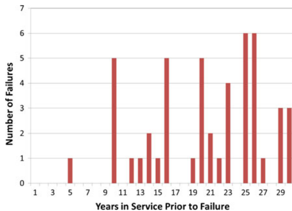
Fig. 1 Distribution of MV power cable failures with respect to years to failure from NEI survey of existing NPPs [1]
