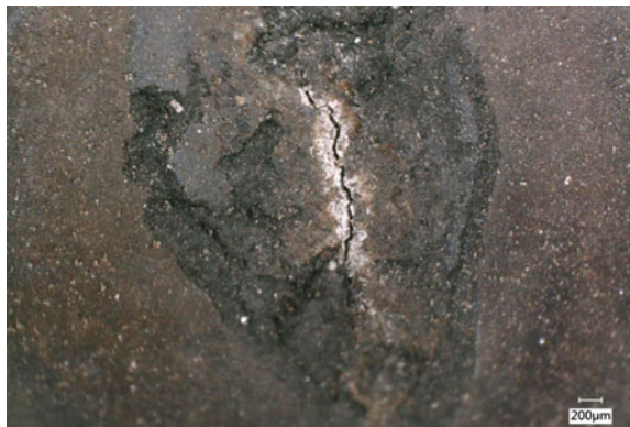
Fig. 13 Higher magnification view of the through-wall leak location
