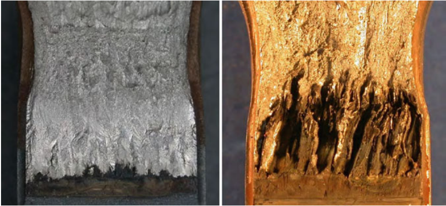
Fig. 4 Macro photographs of 0.5TCT Alloy 82 SAW specimen c764 (left) and 0.5TCT Alloy 82 MIG specimen c765 (right)
