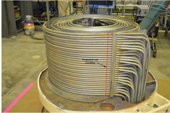
Fig. 3 The letdown cooler after shell removal. The cut location to isolate the tubes is indicated
