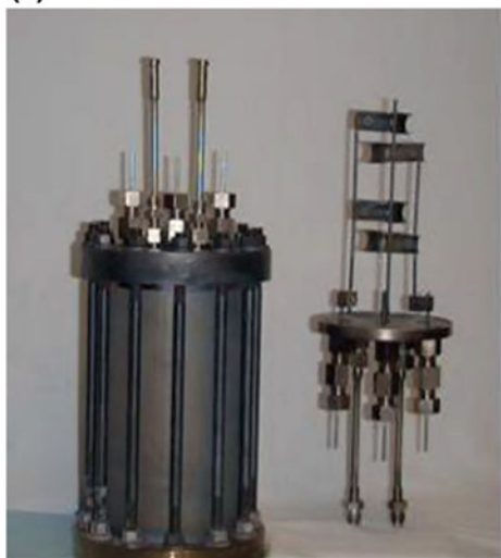
Fig. 1 a Autoclave and mount (shown upside down) for RUB specimens for applied ECP tests and b mount for inhibitors testing
