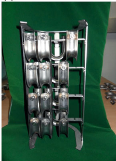
Fig. 1 a Autoclave and mount (shown upside down) for RUB specimens for applied ECP tests and b mount for inhibitors testing
