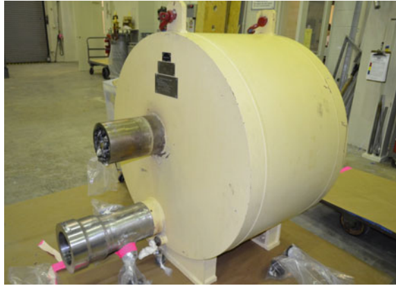
Fig. 1 Receipt photograph showing the primary flow seal side of the letdown cooler. The primary inlet (near center) and outlet (toward bottom) manifolds are visible
