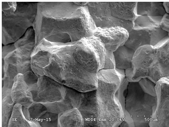
Fig. 17 SEM image of the opened crack taken in the mid-wall region
