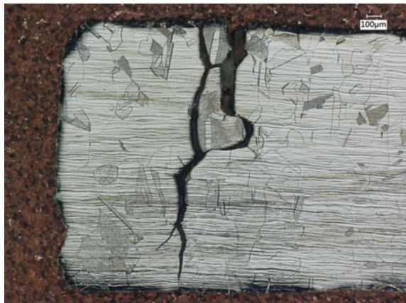
Fig. 25 Same area as Fig. 24, after etching per ASTM A 262, Practice A. No evidence of ditching was noted at the grain boundaries
