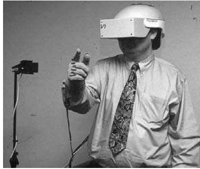
Figure 10.5. Virtual reality immersion helmet with movement-sensitive glove
