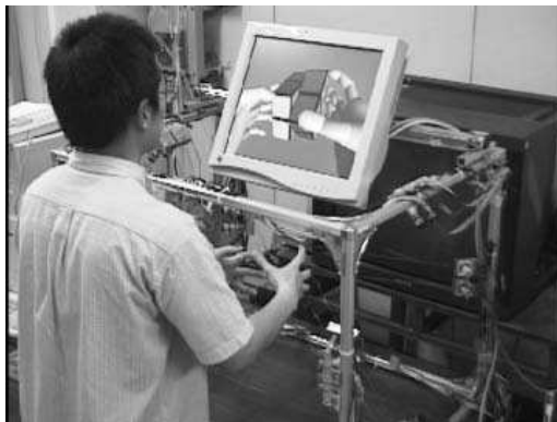
Figure 10.6. Force-feedback mechanical interface, the Spidar 8 (photo: PIL)
