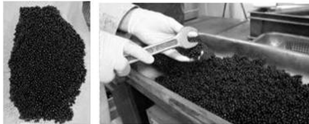
Figure 12.16 Hammering the cooled artificial RA to loosen the particles at 15 °C.
