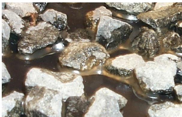
Figure 13.15 A photograph demonstrating rapid wicking of water on the aggregate surface immediately after placed on the CRS asphalt emulsion.
