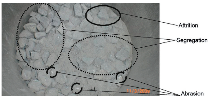
Figure 14.6 Example of attrition, segregation, and abrasion phenomena observed at 100 gyrations using the gyratory shear compactator.
