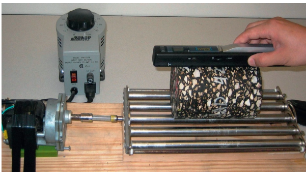
Figure 8.3 Digital lateral scanner (i.e., hot-dog tester) of an asphalt mixture sample.
