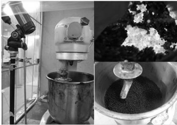
Figure 12.15 Mixer setups and thermography of a mixture.
