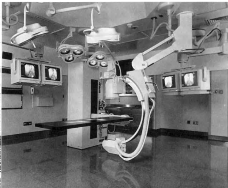
FIGURE 21.4. A ceiling-mounted surgical C-arm roentgenographic unit with image enhancer and a nonmetallic, carbon fiber surgical table are vital components of today's vascular intervention surgical suite. The table, supported by a telescoping pedestal at one end, provides complete clearance beneath for the mobile C-arm and allows vertical travel from 28 to 48 inches, 20° side-to-side roll, and 20° Trendelenburg tilt (standard and reverse). Monitor screens are conveniently mounted for easy visibility.
