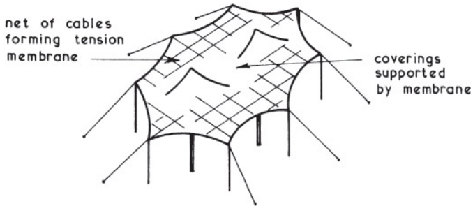
TENSION MEMBRANE STRUCTURE
