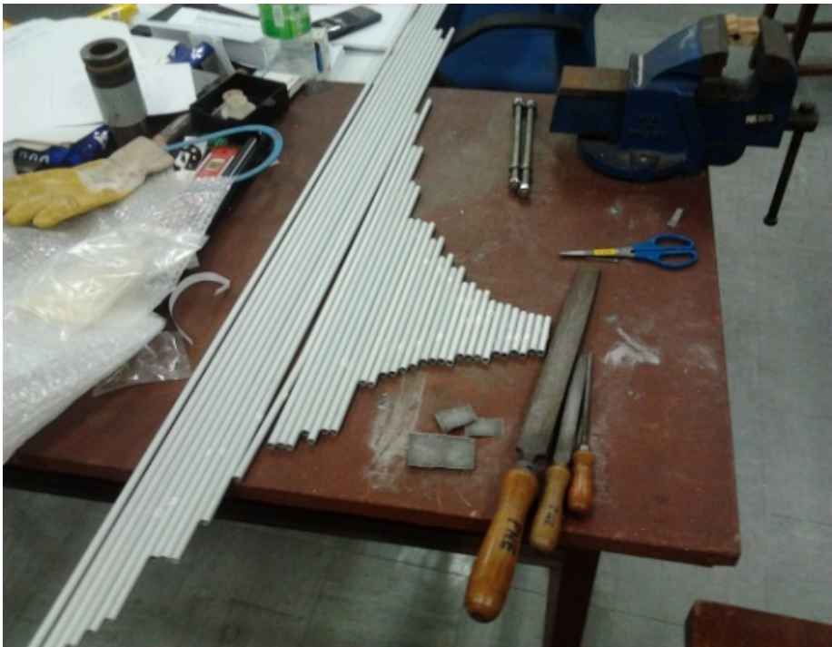
Fig. 1. Preparation of construction of LPDA
