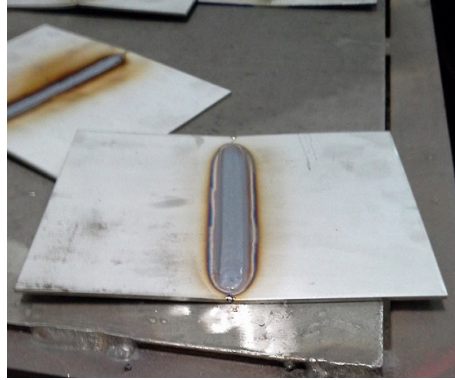
Fig. 1. Butt joint welded workpiece from a single pass
