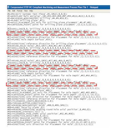
Figure 11.15. Generation of compensated STEP-NC compliant machining and measurement process plan
