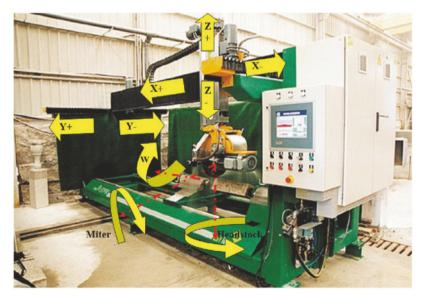
Figure 6.1. Six-axis circular sawblade stone cutting machine
