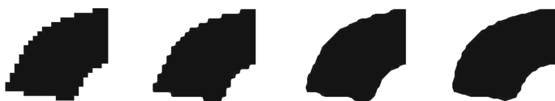
Fig. 4. Enlarged parts of images from Fig. 3 – original image and median sets with the size of B equal to 10 (left), 20 (middle), 30 (right)
