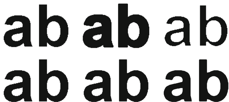
Fig. 3. An application of erosion-dilation median set to binary image enlargement. On the top: left – original image; -middle – dilation; - right – erosion. Bottom row – medians with the size of B equal to 10 (left), 20 (middle), 30 (right)
