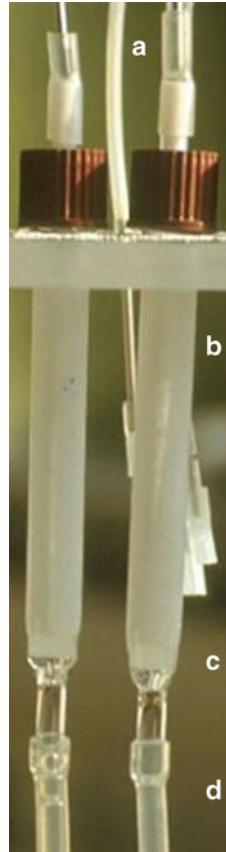
Fig. 1 Glass columns filled with PFA-Teflon beads for hydrophobic interaction chromatography of bacterial suspensions: a inflow tube, b glass column filled with PFA-Teflon, c glass frit to separate column bed from outflow, d outflow
