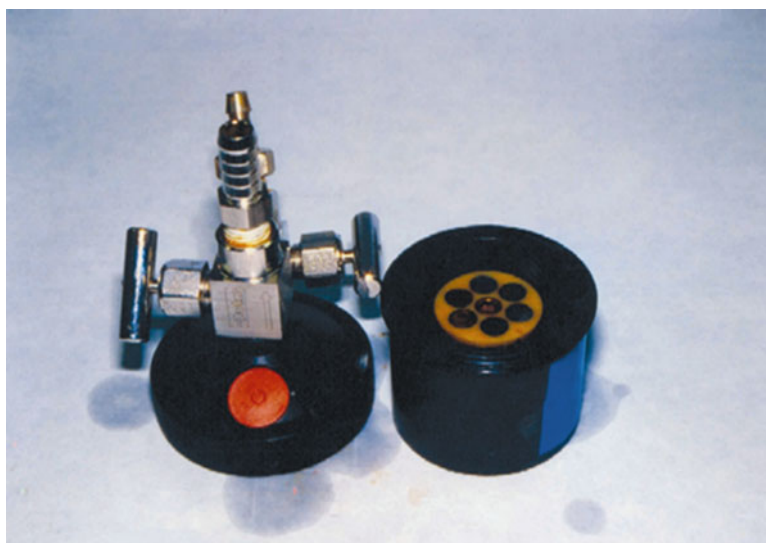
Fig. 2 The picture shows a transport container for biocoupons. The biocoupon housing is mounted and secured in the container by a central corrosion-resistant screw. The container and lid is closed by screw threads. After closing the container, anoxic sample water is carefully flushed through the valves before they are closed
