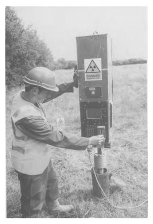
**Fig. 3.22.** Borehole logging systems are now available which are self-contained, incorporating a winch, sonde and recording device and which can be mounted on the borehole. This enables the logging to be undertaken either by the geologist or geophysicist or by the driller himself. (Courtesy of BEL Geophysical Ltd.)
