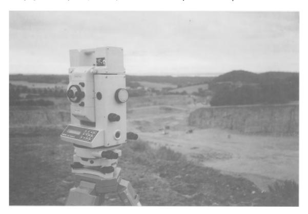
**Fig. 3.6.** Modern topographical surveying equipment can record all survey data digitally. When downloaded into a computer, this enables topographical maps to be prepared rapidly and efficiently, and also allows survey data to be passed directly to geographical and mining assessment software. (Courtesy of West Country Surveys).
