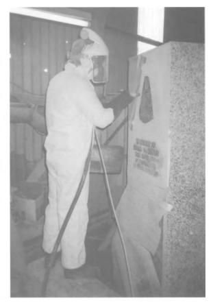
**Fig. 6.33.** Engraving a monument by grit blasting (Courtesy of Natural Stone Products Ltd).
