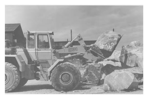
Fig. 5.48. Wheeled loader with fork attachment carrying a block (Courtesy of Realstone Ltd).
