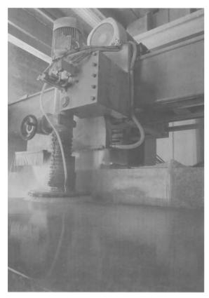
Fig. 6.18. Block cutting or stabbing saw (Courtesy of SEA Diamond Tools).
