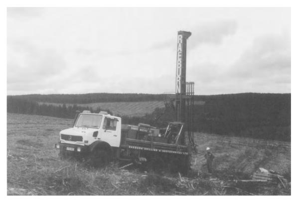
Fig. 3.13. A modern drilling rig, mounted on an all-terrain vehicle, drilling a borehole in a potential dimension stone deposit in Scotland.
