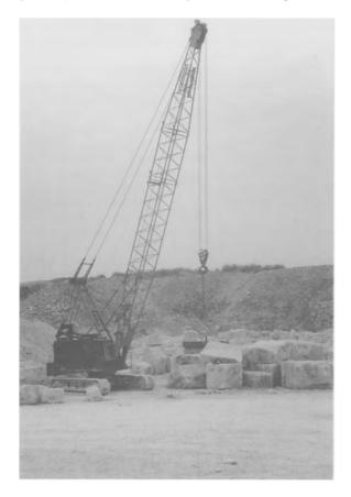
Fig. 5.49. Crawler crane (Courtesy of ARC Ltd).
