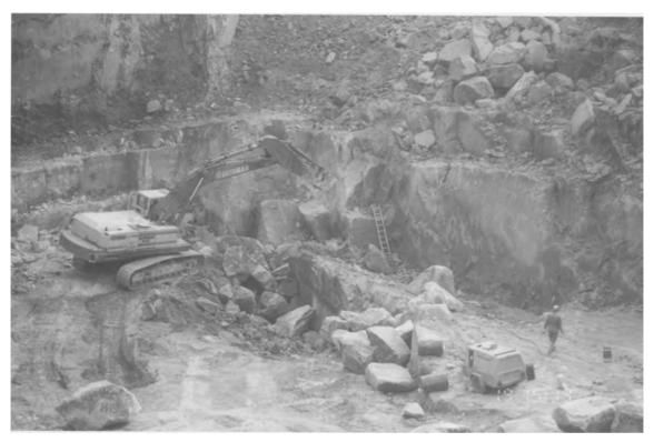
Fig. 6.49. Hydraulic claw removing a sandstone block from Birchover quarry (Courtesy of Natural Stone Products Ltd).
