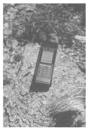
Fig. 3.7. A hand-held GPS system being used to locate boreholes in an exploration site in the Caribbean.
