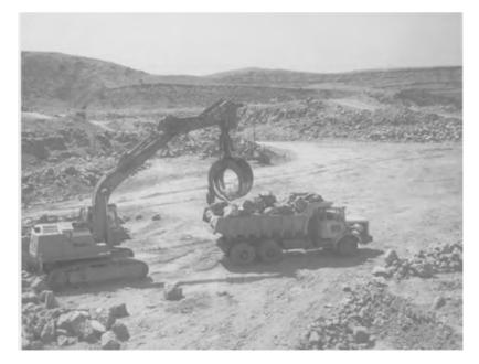
Fig. 8.13. Loading of armourstone blocks into a truck for bulk weighing.
