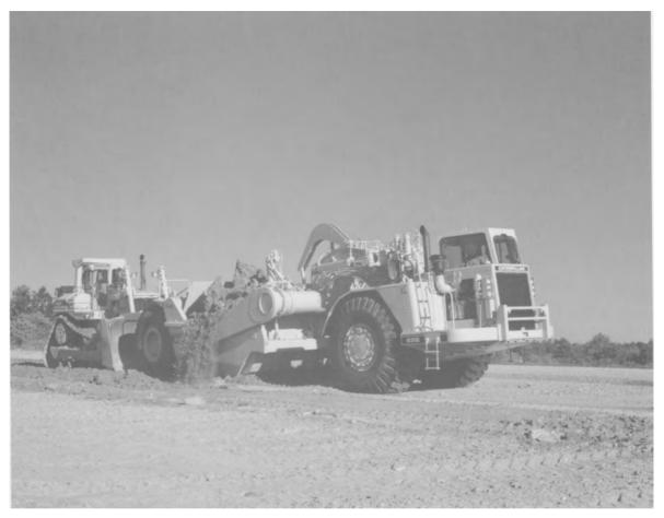
Fig. 5.30. Scraper assisted by tractor bulldozer removing soil (Courtesy of Caterpillar).
