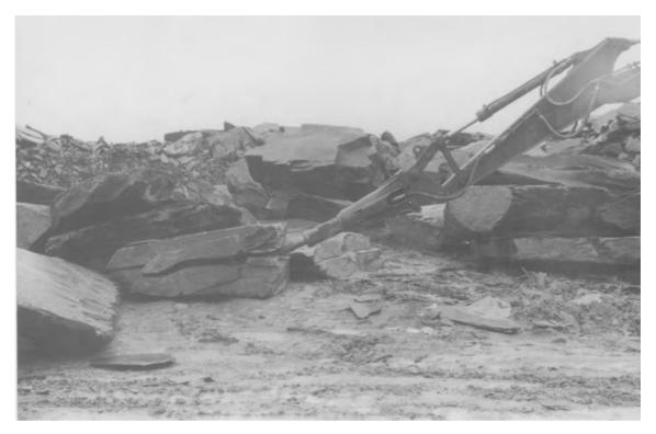
Fig. 6.44. Hydraulic pick splitting blocks of slate (Courtesy of Alfred McAlpine Slate Products Ltd).
