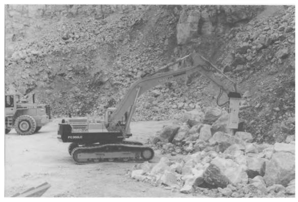
Fig. 6.1. Hydraulic hammer attached to an hydraulic excavator.
