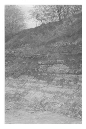
**Fig. 3.5.** The 'Silver Bed' and other building stone, seen at the base of the face in Lincoln Cathedral quarry, is overlain by a sequence of limestones and shales. When this overburden is being removed the thicker limestones are separated and stockpiled in order that the stone can be hand-dressed for use as walling stone.
