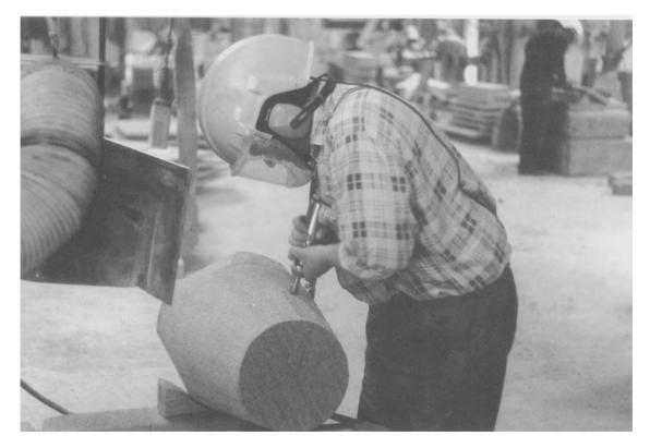
Fig. 5.6. Dolly pointing of a granite bollard by operator wearing an 'Airstream' helmet (Courtesy of Natural Stone Products Ltd).
