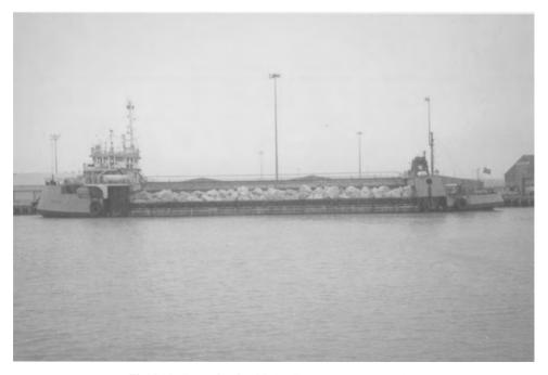
Fig. 8.15. Example of a side loading armourstone carrier.
