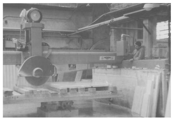
Fig. 6.14. Photograph of secondary, circular diamond saw supported by a fixed bridge.
