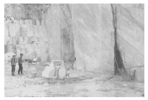
Fig. 5.42. Diamond wire saw in a Greek marble quarry.
