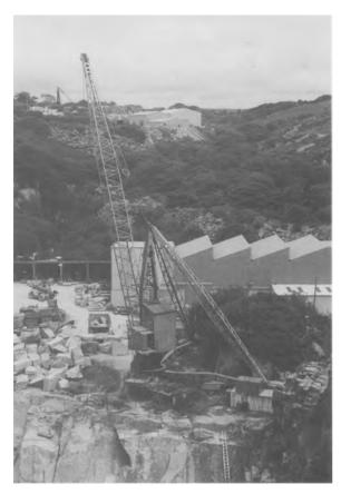
Fig. 5.56. Derrick crane with stiff-legs (Courtesy of Natural Stone Products Ltd).
