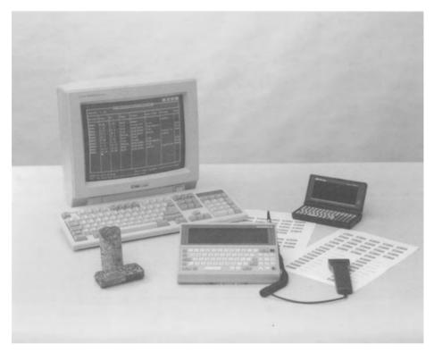
Fig. 3.9. Field data-capture systems, using bar-code readers and notebook computers are becoming common, especially where computer systems are used to process the field data. (Courtesy Field Data Systems Ltd.)
