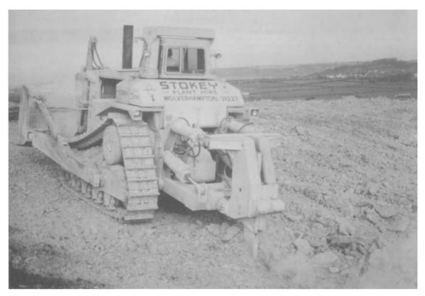
Fig. 5.31. Crawler tractor fitted with ripper (Courtesy of Caterpillar).
