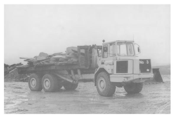
Fig. 6.45. Articulated truck fitted with flat-bed to carry slate blocks (Courtesy of Alfred McAlpine Slate Products Ltd).
