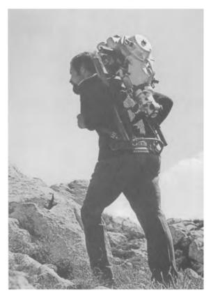
**Fig. 3.8.** Lightweight and even hand-held drilling machines are available for sampling during reconnaissance surveys (Courtesy Atlas Copco).
