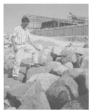
**Fig. 8.12.** Individually weighed 0.3 tonne granite armourstone blocks, rejected by quality control inspector because of poor shape or incipient flaws.
