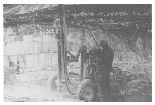
Fig. 5.45. Drilling a vertical hole for a wire saw in marble.
