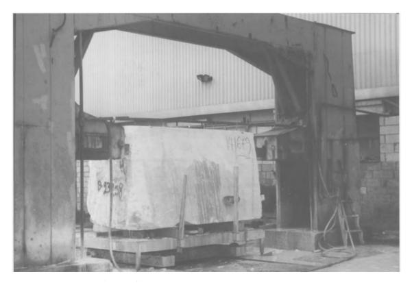
Fig. 6.12. Single blade frame saw cutting a marble block.
