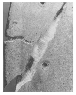
Fig. 9.35. Disruption of natural stone as a result of the formation of ice.
