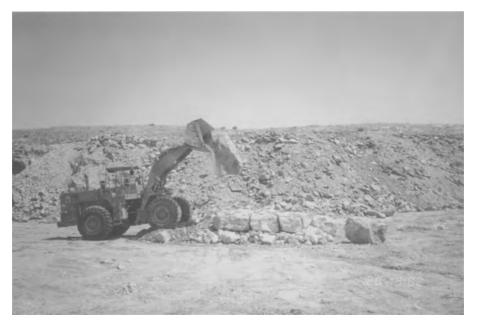
Fig. 8.22. Example of a drop test in an Omani quarry.
