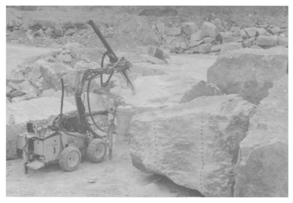
Fig. 5.27. Hydraulic, top hammer drill rig (Courtesy of ARC Ltd).
