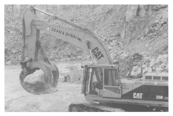
Fig. 6.4. Handling armourstone by mechanical tongs fitted to a hydraulic excavator.
