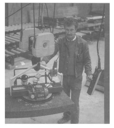
Fig. 6.8. Vacuum cup device handling a stone slab (Courtesy of Vacustonelift).
