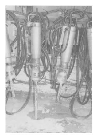
Fig. 5.37. Hydraulic splitters (Courtesy of ARC Ltd).
