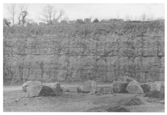
Fig. 5.18. Presplit face showing half-barrels (Courtesy of RMC Roadstone Ltd).
