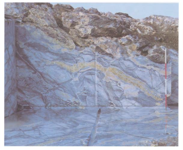
Fig. 4.2. The variation in the colours of Ledmore marble is produced by variations in the mineralogy. (Photo courtesy of Fife Silia Sands Ltd.)
