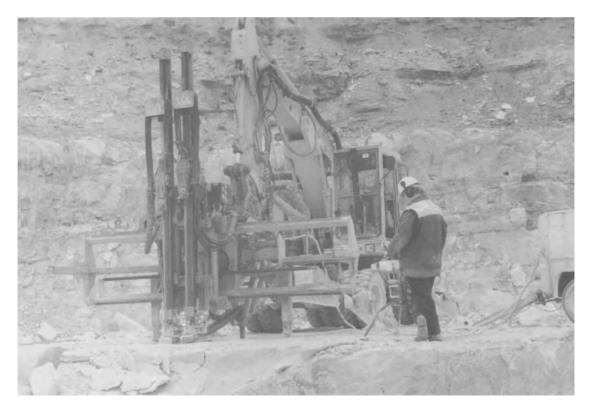
Fig. 5.67. Quarry bar supporting two top-hammer drills (Courtesy of ARC Ltd).
