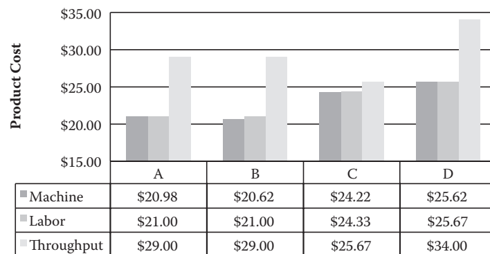
Figure 7.2 Comparison of standard costing (machine and labor allocations) and throughput methods.
