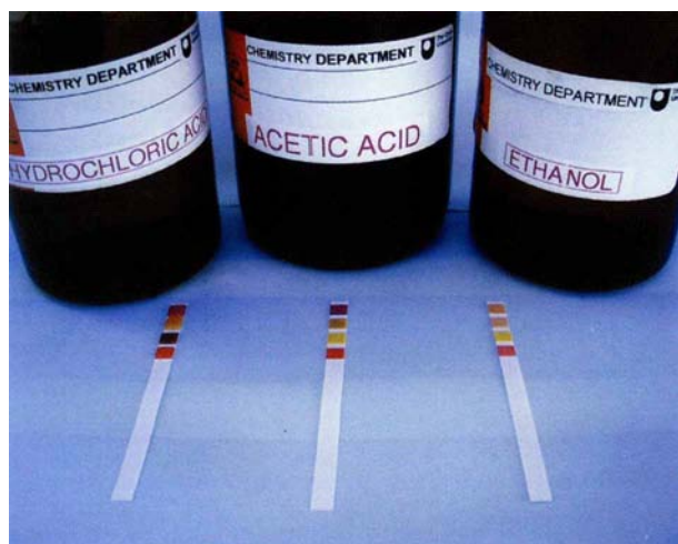
Figure 3.4 pH papers can be used to measure the pH of an aqueous solution of hydrochloric acid, ethanoic acid (acetic acid) and ethanol. The results are pH 1, pH 4 and pH 7 respectively.
