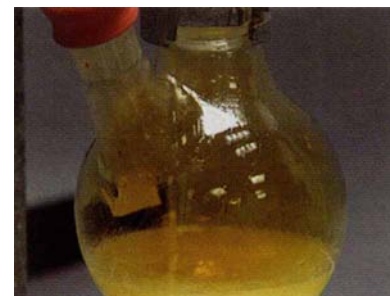
Figure 3.1 The reaction of benzene with nitric acid: brown fumes of NO 2 are formed as a by-product.
