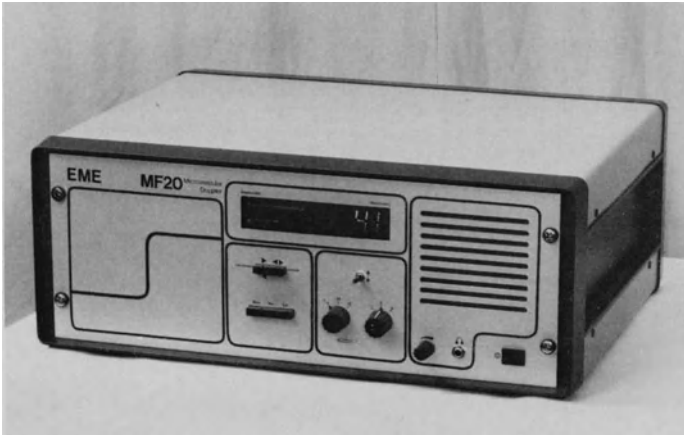
Fig. 9. The present appearance of the microvascular Doppler system MF 20 (original name of the prototype: Microflo) Eden Medizinische Elektronik GmbH, D-7770 Überlingen
