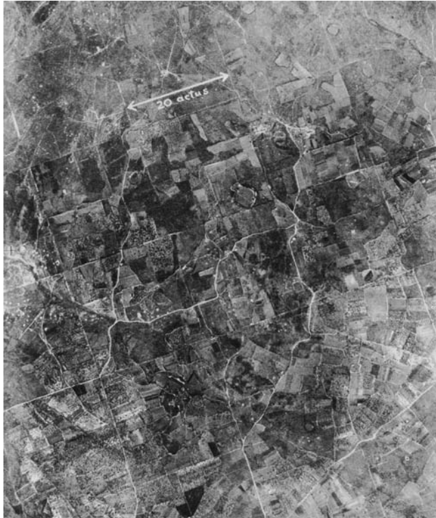
Figure 16.2 Checkerboard pattern of Roman land division (“centuriation”) as seen from the air near modern Pula (Croatia) in the Istria peninsula. ( Barrington Atlas map 20A5.) Roads form an integral component. The basic unit here is typical, square in shape, with each side 20 Roman actus in length (= approximately 700 meters). J. Bradford, Ancient Landscapes: Studies in Field Archaeology . London, 1957, plate 40; reproduced by license from UK Office of Public Sector Information
