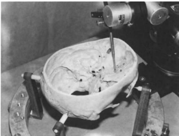
Fig. 2. A metal target glued on a dry skull, touched with a probe mounted on the toolholder. Skull has been previously scanned, with a CT localizer mounted on the stereotactic frame
