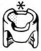
Fig. 8.52 Cross-link sleeve with a section cut away* allowing a range of angulation of the cross-link rod (see Fig. 8.6)
