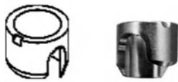
Fig. 8.23 Sleeve with short and long legs, small mark on the top of short leg.
