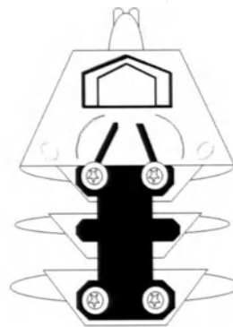
Fig. 2.8 This constrained system with locking screws allows unicortical purchase
