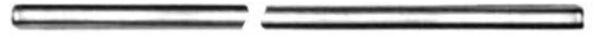
Fig. 8.122 6 mm rod comes in two different types: soft rod, length 50–150 mm; hard rod, length 200–500 mm
