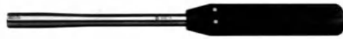
Fig. 8.112 Socket wrench with a spring mechanism at the bottom to hold the sleeve and nut in place
