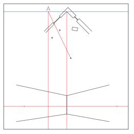
$9^{\text{To}}$  obtain vertical information, you must follow a two-step process. Draw a construction line that intersects the SP and any point on the plan and continue it through the PP (label A at the PP).
