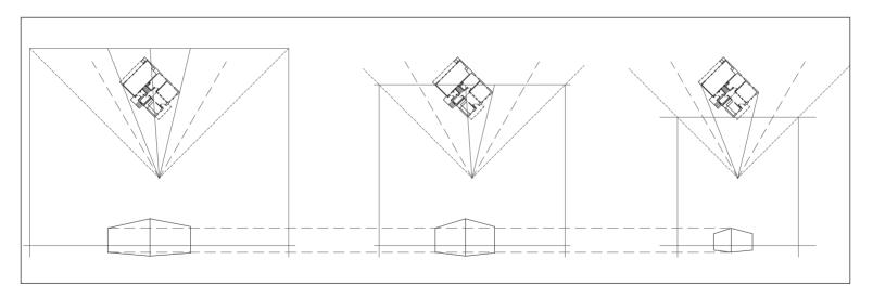
▲ **Moving picture plane** The location of the PP determines the relative distance between the vanishing points (VPs). As the PP moves away from the SP, the VP move apart. Where the PP crosses the plan determines the location of the ML. If the ML is constructed off the front of the plan, then the image recedes to the back. If the ML is constructed off the back of the plan, the image will project forward.
