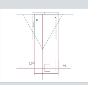
$4^{\text{Construct the back wall elevation that corresponds to the}_{\text{Iocation of the PP at the same scale as the plan. Draw this}_{\text{in the open space below the plan. This will serve as your ML,}_{\text{or in this case your measuring plane (MP).}}$
