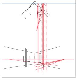
1 3 All vertical measurements must be translated along Surfaces if they do not connect directly to the ML (such as the chest in this drawing). That is, an object detatched from a wall touching the ML must have its vertical measurements transferred across a series of perpendicular planes (even if those planes do not exist as actual surfaces in the design).
