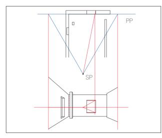
$9 \ {\rm Show}$  the depth of the wall at the window opening. Extend a line from the SP through a point on the plan to where it crosses the PP and drop a vertical line down. Use measurements from the MP to draw the corners receding to the VP.
