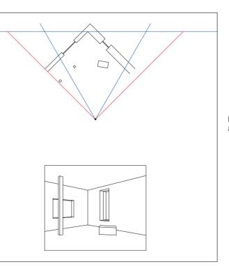
1 4 Finished perspective. The CV (shown here in blue) establishes the box around the perspective.
