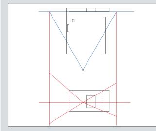
$5^{\rm Start}$  the drawing by connecting the VP to each of the four corners of the elevation. Extend these lines beyond the limits of the elevation. This will provide the parameters of the room: walls, floor, and ceiling.
