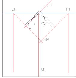
$5^{\rm Label}$  the intersections of lines L and R with the PP L1 and R1. At R1, the intersection of the construction line and the PP, draw a vertical construction line, perpendicular to the PP into the open space of the page. Repeat at L1.
