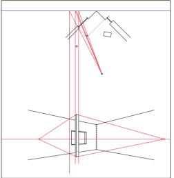
$1\,1$  Go back and forth between getting vertical information from the plan, measurements from the ML and surfaces that vanish to one of the VPs. Heights can only be taken along assisting planes for elements not along the ML. See "assisting planes," page 93.
