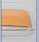
**1** Soak the basswood in water until the material is completely saturated—about 30 minutes.
