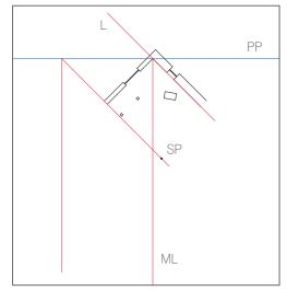
**4** To determine the location of the vanishing points it is important to follow these instructions exactly. From the SP, and using your adjustable triangle, draw a construction line parallel to line L of the plan that intersects the SP and crosses through the PP. Repeat on the other side for R.
