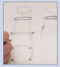
Buse an HB lead to begin to darken in the delements that are cut in section. Section cuts are continuous and shall not be left open-ended. Make crisp dark lines with a sharp lead. The light construction lines should remain on the drawing.
