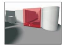
▲ **Spatial diagrams** Similar to the axonometric diagrams, these perspectival digital spatial diagrams depict the apparent and implied spaces that are formed after two new elements are inserted into an existing context. CASE STUDY: 3
