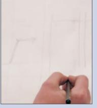
**1** Use a 4H lead to create a series of construction lines to establish the boundaries of the chair. Determine the chair's width proportion to its overall height. Continue to establish these proportions for all of the required orthographic projections. Complete this step before adding detail and line weights.
