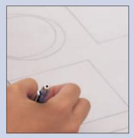
$\label{eq:sure} \begin{array}{l} 3 \\ \text{Sure that the line weights in one elevation} \\ \text{match the line weights for all the elevations on} \\ \text{the same page. Consistency is important.} \end{array}$
