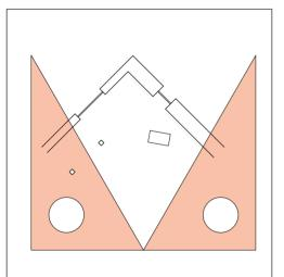
**1** Use two 30/60/90 degree triangles to establish the cone of vision. The point of the two triangles indicates the location of the SP. Tape down the plan and lay a large piece of trace or vellum overtop. Place the sheet of paper so that it covers the entire plan and leaves room at the bottom for the image.
