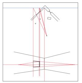
1 Obraw a second construction line, starting at A (the intersection of the first construction line and the PP) perpendicular to the PP into the perspective image area. Repeat for all lines in a given element. Cross the vertical lines with height lines obtained from the ML.
