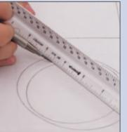
**1** Draw two lines. Take any scale measurement that is divisible by nine. Lay the zero on the left line and the nine on the right. Mark off the corresponding increments of nine to set up evenly spaced increments.
