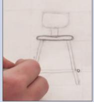
2Use an H lead to begin to darken the elements that are seen in elevation. The construction lines remain the lightest line weight on the page and should, at this point, begin to fade naturally as other, darker, lines appear to become more dominant.
