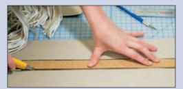
**1** Use your straightedge to cut material. Score first, then make a series of cuts. Do not try to cut the material with one stroke.
