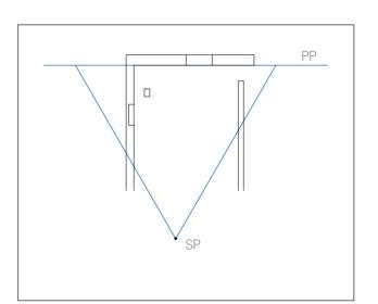
$2^{\mbox{Draw}}$  the PP to coincide with the back elevation for ease of construction. That is, the horizontal line demarcating the PP should cross the front edge of the wall. Blue lines indicate the cone of vision (CV).
