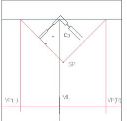
Twhere the vertical lines from the PP cross the horizon line, you will establish the vanishing points. Call them VP(R) and VP(L). The ML should also cross the horizon line. This intersection establishes the location of the eye level for the person standing at the SP. If the person is standing on the ground, the horizon line would be 5 ft (1.52 m).
