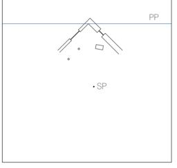
$2^{\text{Next, establish the location of the picture plane (PP). For} \\ \text{Point on the plan, preferably a corner of the plan and one that} \\ \text{will be seen in the perspective image.}$
