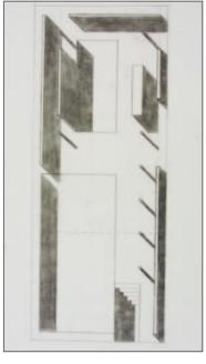
▲ Indication of depth in plan Shadow plans indicate the changing floor depths. They reveal the relative heights of individual elements and the relationship between solid and transparent surfaces.
