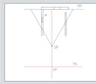
**3** Locate your HL and VP on the elevation. The VP should correspond to the appropriate height of a viewer's eyes looking into the space and can be located directly in line with your SP. The SP and VP vertically align since this is a single-view perspective with one focus.
