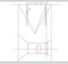
$6^{\mbox{Vertical lines are obtained through the same method as}$  the 2-point perspective (see page 90). Method: SP to the point on the plan; where the line crosses the PP drop a vertical line down.
