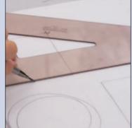
$2^{\text{Make sure to lift your triangle after}}_{\text{making vertical lines to avoid smudging}}_{\text{the drawing.}}$
