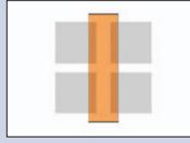
A series of overlapping boxes indicates a subtle connection between two elements: circulation (orange) and classroom units (gray). This diagram describes how these units can overlap into the hallway as instructional areas.
