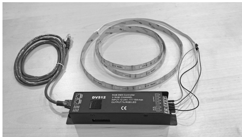
Figure 9.11 This is a DMX LED Lighting controller that can be attached to a DMX-512 network.
