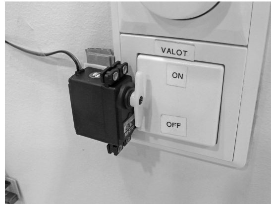
(b) A servo motor mounted over a light switch, which was used to turn the lights on and off in the room.
