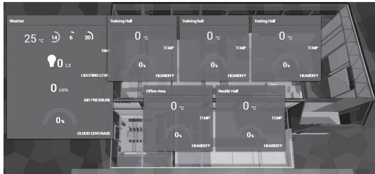
(b) Screen shot of a web interface used to show the values from sensors throughout an industrial facility.
