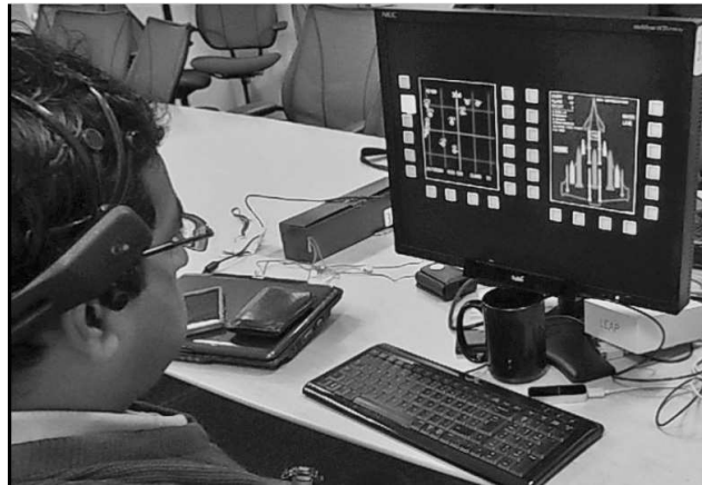
Figure 10.4 Hands-free pointing using head-tracking or eye-gaze can be included as a possible interaction modality for aircraft cockpit multi-function displays.
