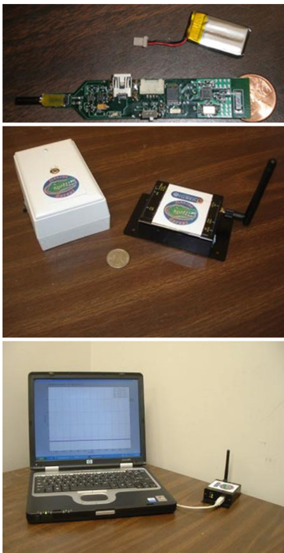
Fig. 10.11 Photographs of integrated pH sensor ( top ) and receiver/transmitter pair ( center ) and connection to computer (bottom)
