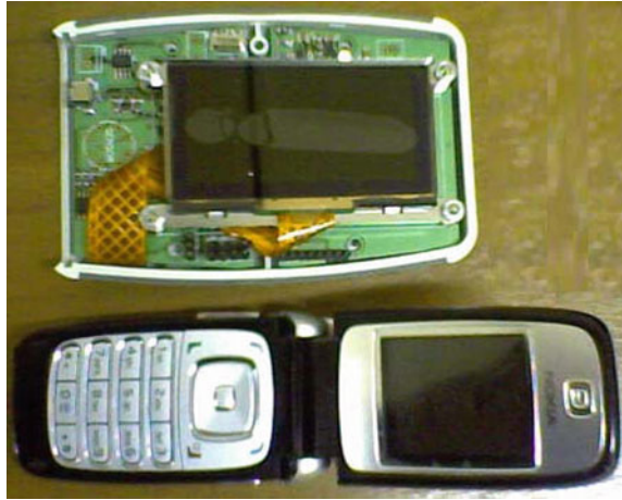
Fig. 9.18 Prototype of a compact chemical sensor that is incorporated into a mobile phone. Courtesy of Dr. Francisco Hernandez-Ramirez
