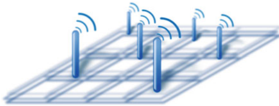
Fig. 13.28 Sensor grid consisting of several individual sensor nodes, interacting via wireless data links. Such sensor grids can provide real-time images of the air contamination inside buildings, air cabins and/or heavily populated city environments
