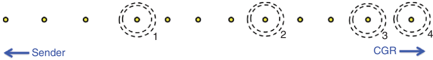
Figure 9.3 Pictorial proof idea showing why SAGP only uses O(\lg n) transmissions per geocast in dense scenarios. The originator is somewhere to the left of the diagram; the intuition is that, on average, successive transmissions will occur at devices approximately half way to the CGR.
