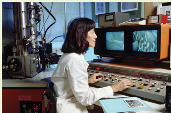
Typical SEM-EDS system. (Lawrence Migdale/Photo Researchers, Inc.)
