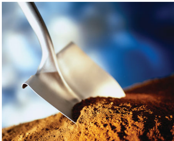
The rolled-over steel flange used to press a shovel into the soil takes an excellent horizontal soil sample. (Corbis)
