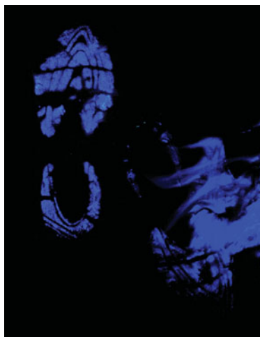
Luminol lights up the traces of blood left after the commission of a crime, even after attempts are made to clean up the evidence. (Courtesy of Michael E. Stapleton/Stapleton Associates, LLC)
