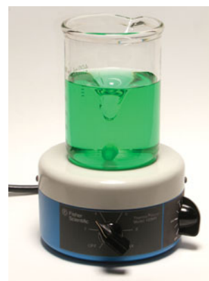
Solutions are stirred and heated to increase the rate of dissolution. (Tom Pantages Stock Photos)
