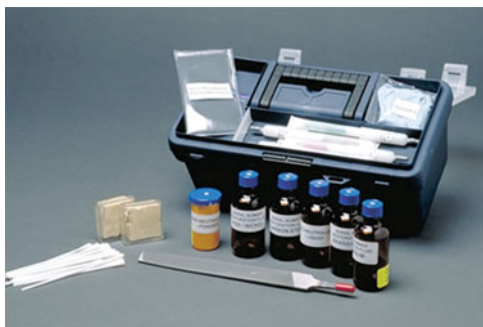
FIGURE 6.4 A serial number restoration kit contains a collection of acid solutions used to restore the serial number etchings on a variety of metal surfaces. (Courtesy Wisconsin Dept. of Justice, Crime Labs Division)
