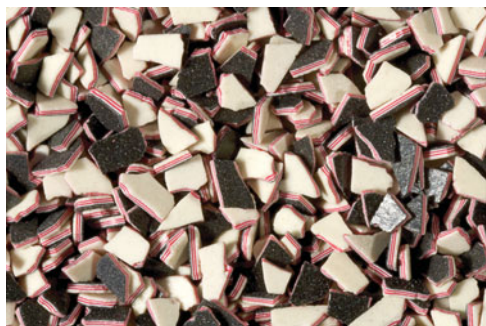
Explosive taggants contain information for identifying the lot number and manufacturer. (Microtrace, LLC, Minneapolis, MN)
