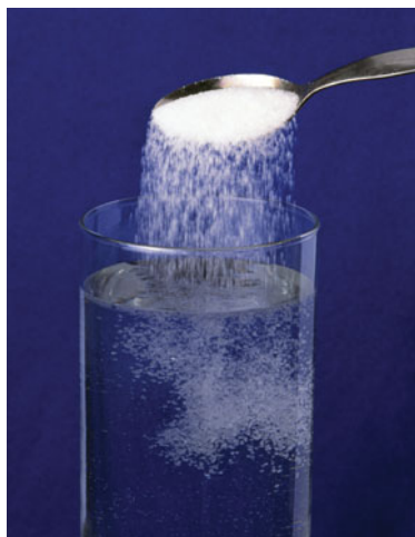
FIGURE 6.1 An aqueous solution forms as the solute (sugar) dissolves into the solvent (water). (Martyn F. Chillmaid/Science Photo Library)
