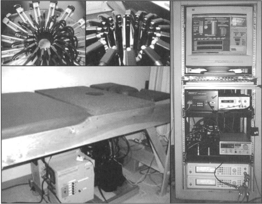
Figure 5. Second-generation system with parallel detection and three layers of optical fibers. The fiber translation array system (top left) drives three layers of fibers (top center) to accommodate radial and vertical positioning relative to the pendant breast. The computer control panel and data acquisition system (right) and the exam table with optical array (bottom left) are also shown. The array of photomultiplier tubes that is translated to multiplex to each of the three layers of 16 detection fibers is immediately below the table.
