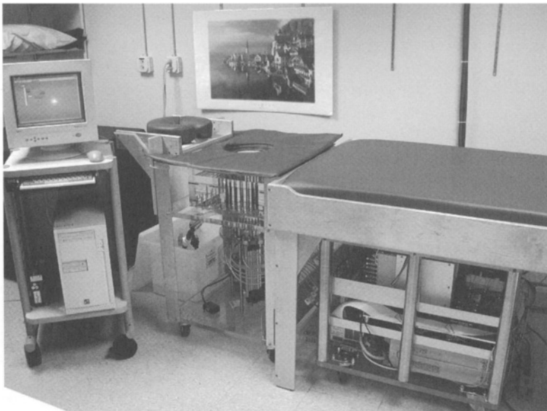
Figure 6. Antennas, illumination tank, and computer-controlled linear actuator assembled on test bench (top) and integrated with breast interface (bottom).
