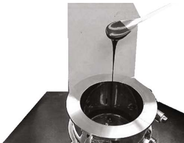
Fig. 7.4 Paint for negative electrodes. 7 Reproduced by permission of CMC Publishing Co. Ltd
