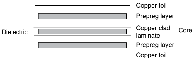
Figure 3.3 A four-layer board layup.
