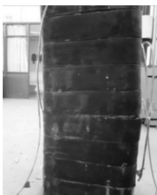
Figure 13. Failure pattern of column SP-3 (before stripping of bands).
