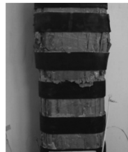
Figure 5. Failure pattern of column DP-3 (before stripping of bands).
