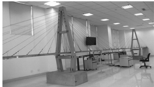
Figure 1. Cable-stayed scale model bridge.
