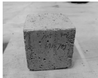
Figure 3. Picture of the M5 specimen with marginal damage.
