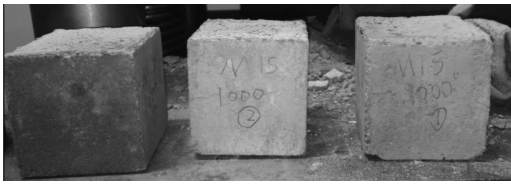
Figure 6. Picture of the M15 specimen with slight cracks.
