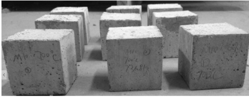
Figure 4. Picture of the M10 specimen with slight cracks.
