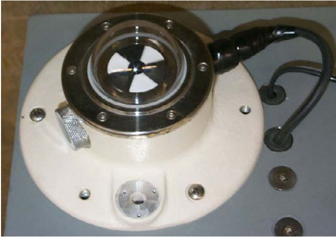
FIG. 10.2. The Eppley pyranometer is typical of the instruments used for the measurement of global, reflected, and diffuse shortwave radiation. The detector is a differential thermopile with the hot-junction receivers blackened and the cold-junction receivers whitened. Temperature-compensation circuitry frees the instrument from the effects of ambient temperature changes. A precision ground optical glass hemisphere of Schott glass (WG295) uniformly transmits energy from 0.285 to 2.800 \mu\text{m} over zenith angles from 0–70°. The sensitivity is 11 microvolts per \text{W m}^{-2} with a response time of 5 s. The size is 5 3/4 in. diameter, 3 3/4 in. high and the weight is 2 lbs.
