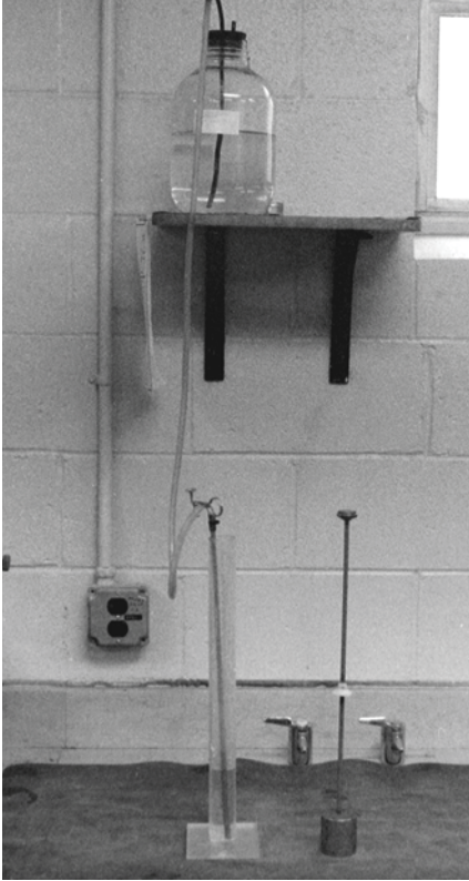
Figure 2 —Graduated Cylinder, Irrigator Tube, Weighted Foot Assembly, and Siphon
