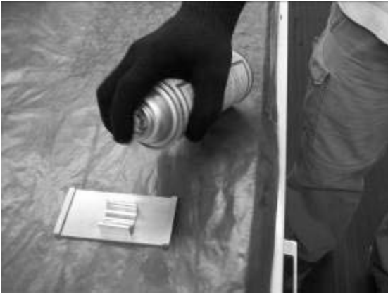
Figure 2 —Spray Release Agent on the Mold
