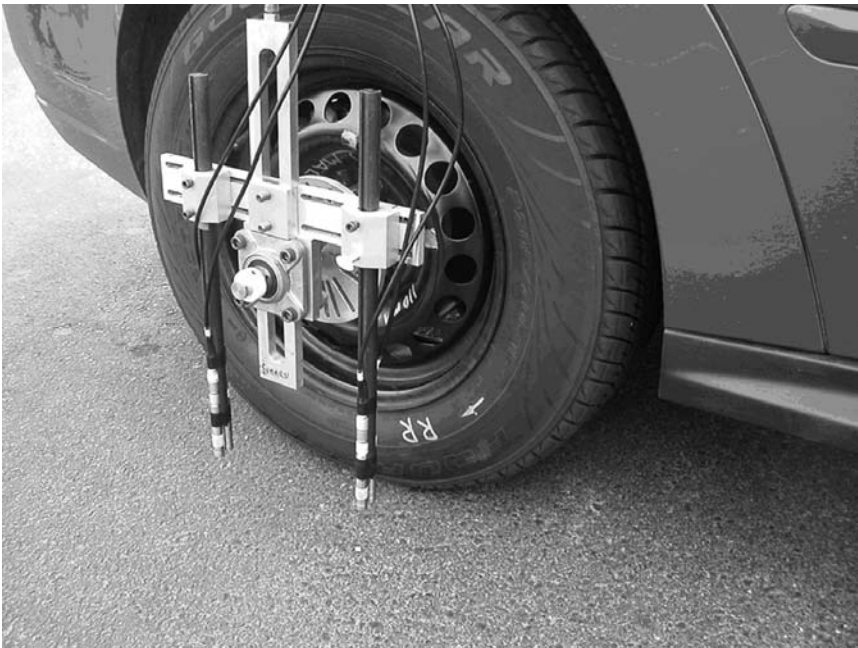
Figure A5.3 —Dual-Probe Vertical OBSI Setup (shown without required windscreens)
