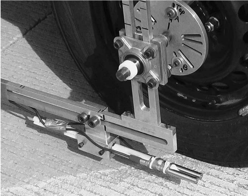
Figure A5.4 —Single-Probe Horizontal OBSI Setup, Leading Edge (shown without required windscreens)
