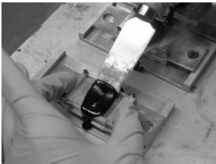
Figure 8 —Trim the Extra Sealant Away Using a Heated Spatula
