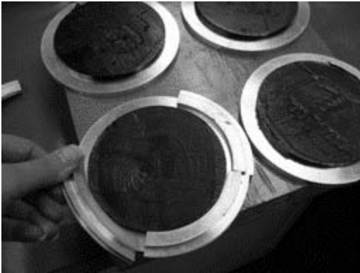
Figure 16 —Removing the Molds
