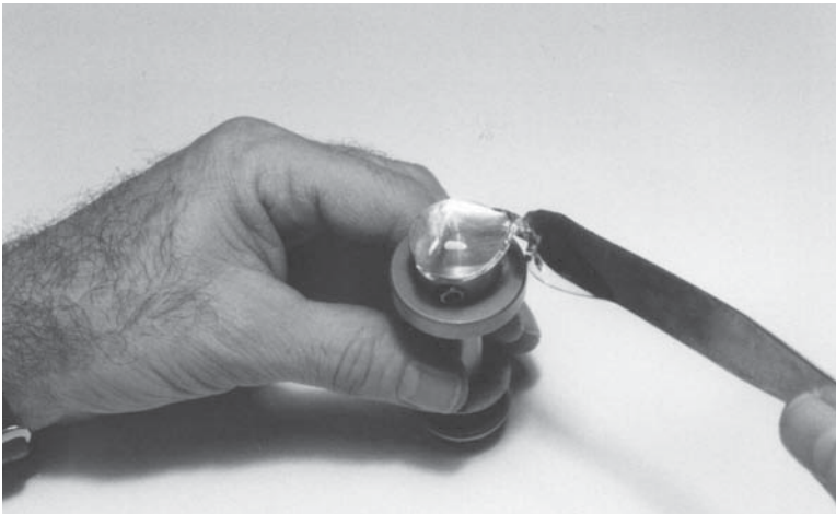
Figure X7.2 —Using a Spatula to Place the Reference Fluid on the Plate
