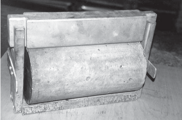
Figure 2 —Jig for Aligning Concrete Cylinder and Bearing Strips
