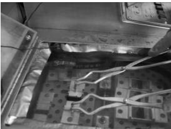
Figure 17 —Grab the Specimen from Two Corners, and Place It Back in the Bath
