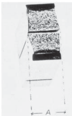
Figure 15 —Halves of Broken Charpy V-Notch Impact Specimen Joined for the Measurement of Lateral Expansion, Dimension A
