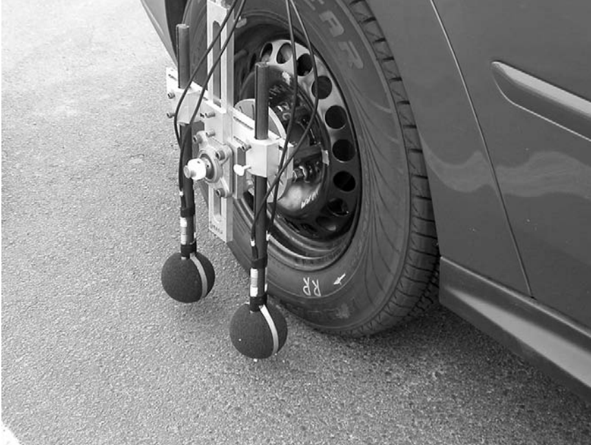
Figure A5.2 —Dual-Probe Vertical OBSI Setup
