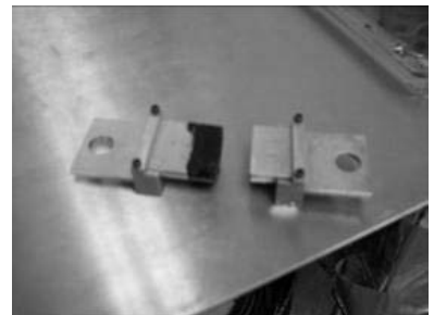
Figure 19 —Turn on the DTT Machine, Load Adhesion Program, Mount the Specimen, Tare the Load to Zero, Run the Test, and Record the Data
