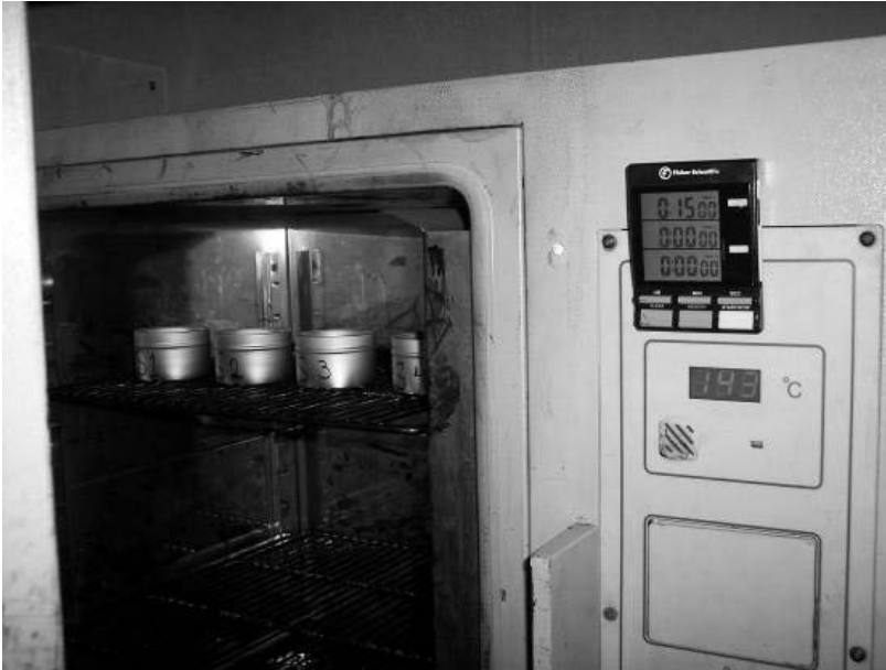
Figure 10 —Heating 35 g of Homogenized Sealant at Recommended Pouring Temperature for 30 min.
