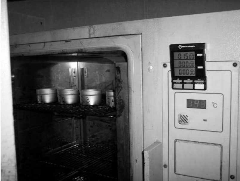
Figure 5 —Heat 35 g of Homogenized Sealant at Recommended Pouring Temperature for 30 minutes.
