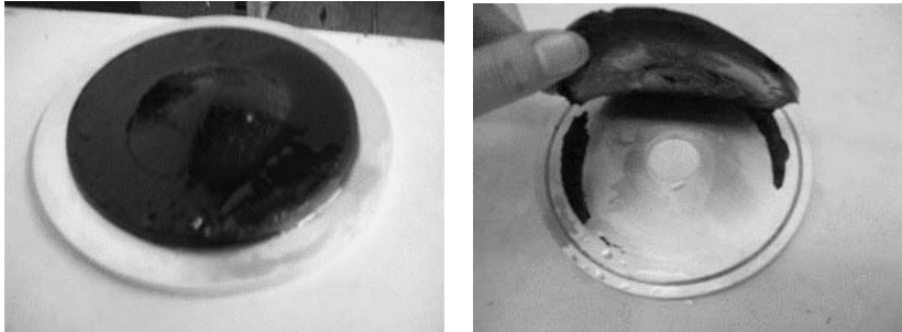
Figure 18 —Removing the Specimen and Verifying that the Type of Failure Was Adhesive Failure, in which Sealant Separates from the Disk
