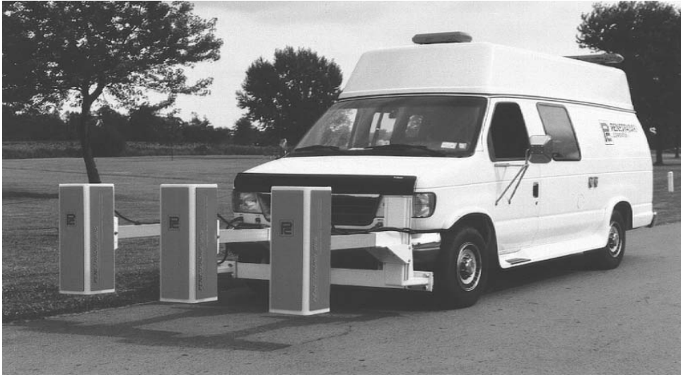
Figure 1 —Multiple Antennae on a GPR Survey Vehicle
