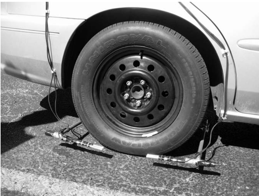
Figure A5.5 —Dual-Probe Horizontal OBSI Setup (shown without required windscreens)
