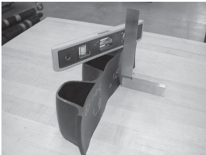
Figure A1.2 —Evaluate the Ends of Milled Specimen with a Carpenter's Square
