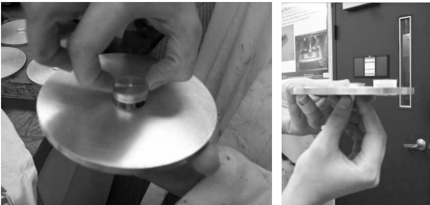
Figure 6 —Placing the Plug on the Annular Disk and Pulling It from Underneath until the Disk Fits in the Orifice and the Film Edges Set on the Disk
