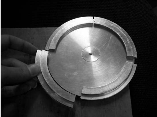
Figure 8 —Assembling the Molds on Top of the Disk
