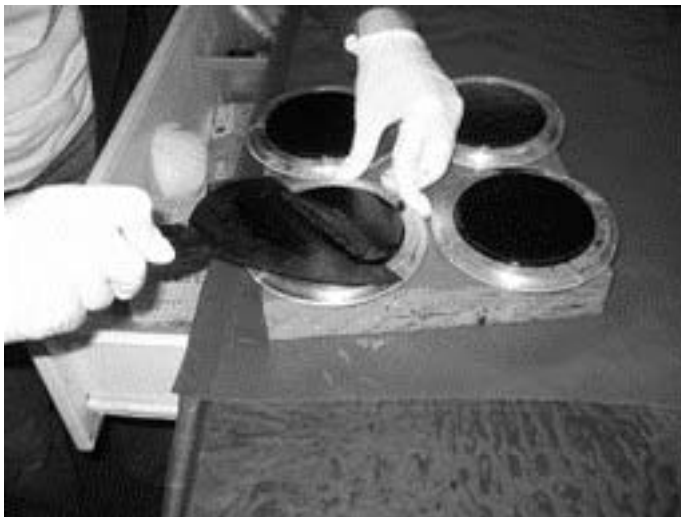
Figure 13 —Trimming Excess Sealant with a Heated Putty Knife
