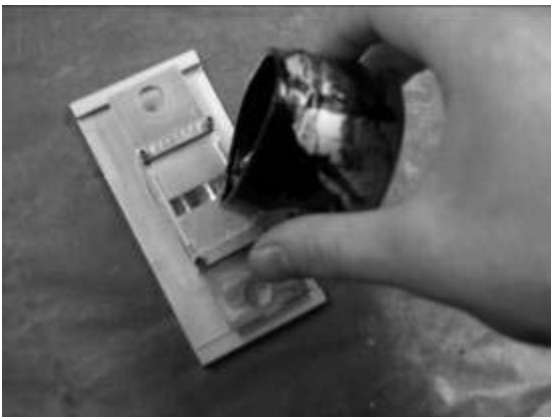
Figure 6 —Remove the Sealant from the Oven, Mix Thoroughly, and Pour It in the Mold from One Corner
