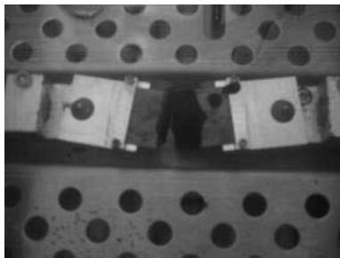
Figure 19 —Turn on the DTT Machine, Load Adhesion Program, Mount the Specimen, Tare the Load to Zero, Run the Test, and Record the Data
