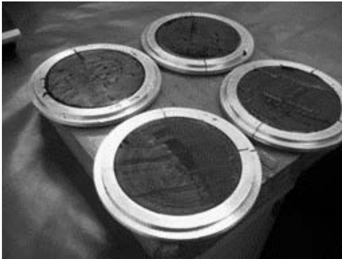
Figure 12 —Sealant Setting for 1 Hour at Room Temperature
