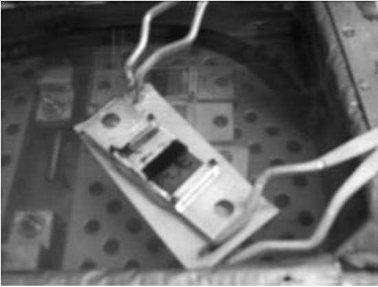
Figure 9 —Grab the Base Plate with Two Tongs, and Place It in Cooling Bath
