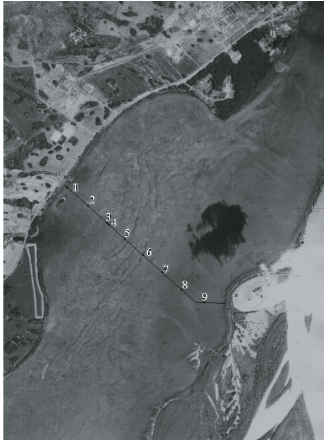
Fig. 9.5 Aerial photograph of the Ob River study site. Upper left , upland with forest patches ( dark gray ) and arable land ( light gray ). Right , the Ob River. Between the upland and the river is the studied fen on the lower Ob River terrace. The dark patch is a cloud. Numbers indicate the locations of piezometers. Note the darker gray peat ridges stretched half-way up the terrace
