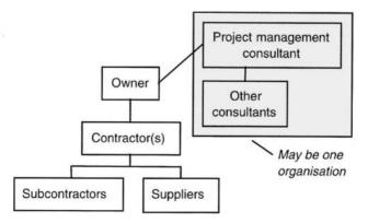
Figure 4.21. Project management method (showing contractual links) - alternative.
