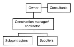
Figure 4.27. Traditional delivery/managing contractor (non-agency) construction management configuration.
