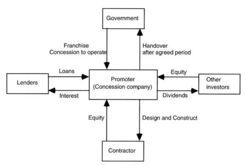
Figure 4.30. Example structure of a concessional scheme.
