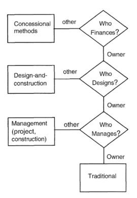
Figure 4.1. Broad discrimination of delivery methods (not all delivery methods are shown).
