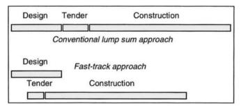
Figure 4.34. Bar chart showing overlap of design and construction phases.
