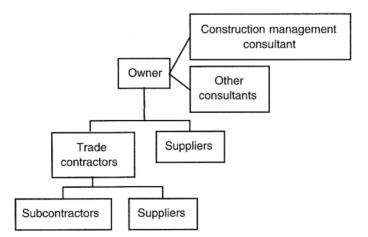
Figure 4.25. Construction management method (showing contractual links).
