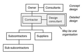
Figure 4.12. Detail design-and-construct method (showing contractual links) – contractor as the lead player. The alternative where the design consultant is the lead player, rather than the contractor, is also possible.
