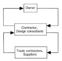
Figure E6b. Project correspondence loop of particular design-and-construct project.
