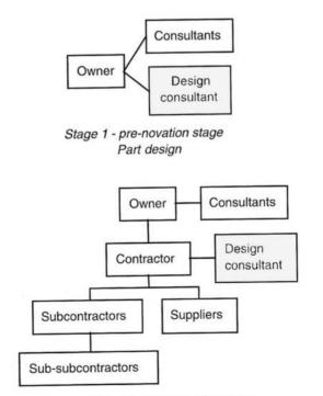
Stage 2 - post novation stage Remaining design plus construction
