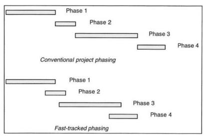
Figure 4.33. Bar chart showing comparison of conventional and fast-track approaches.
