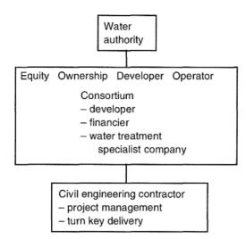
Figure 4.31. Contractual arrangements, water treatment project/plant.
