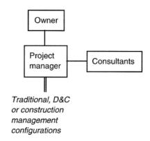
Figure 4.22. Atypical reference to project management method (showing contractual links).
