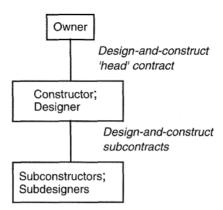
Figure 4.14. Design-and-construct on two levels.
