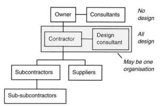
Figure 4.13. Design-and-construct method (showing contractual links). The alternative where the design consultant is the lead player rather than the contractor is also possible.
