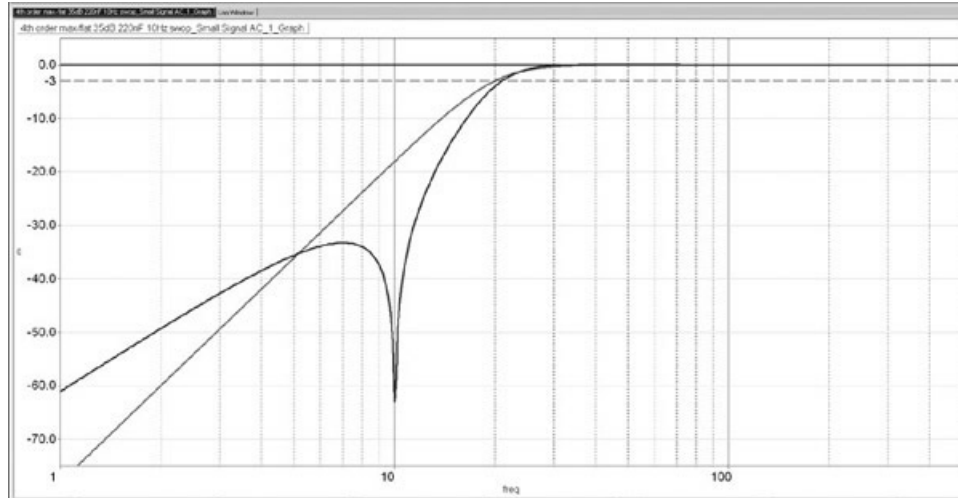
Figure 12.42 Frequency response of 4th-order A_0 = -35 dB classic (non-MCP) highpass elliptical filter that is -3 dB at 21 Hz, almost the same as the 3rd-order Butterworth that is -3 dB at 20 Hz
