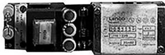
Figure 10.3 The Lenco phono preamplifier
