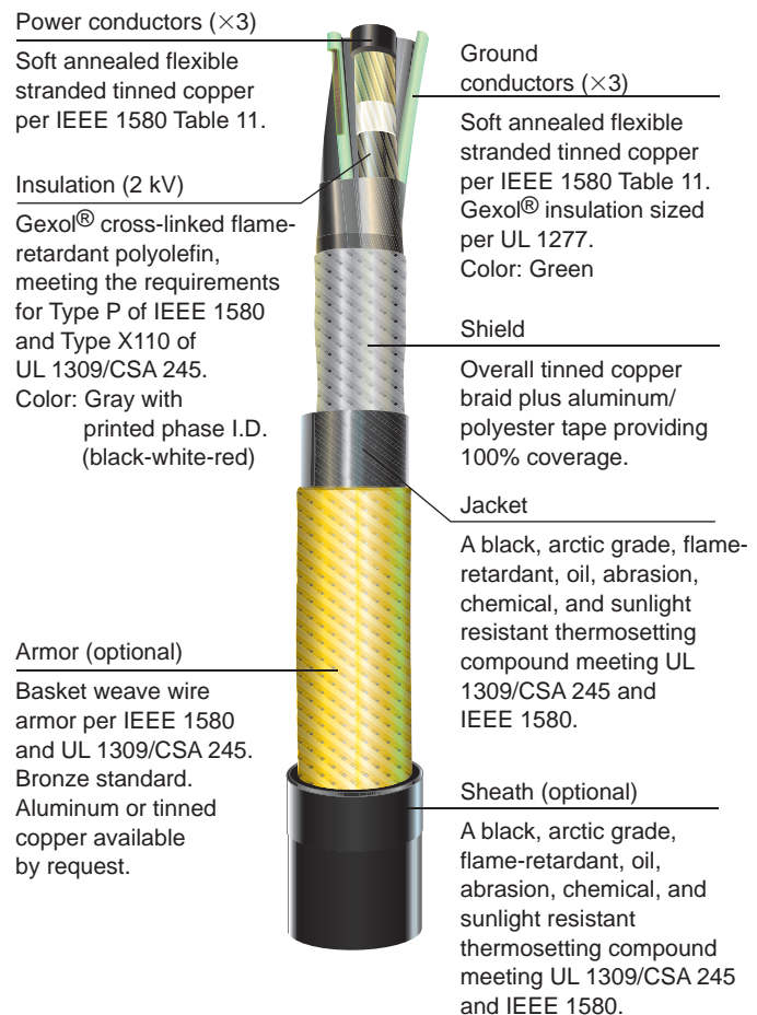
Figure 10-17 VFD shielded power cable.
