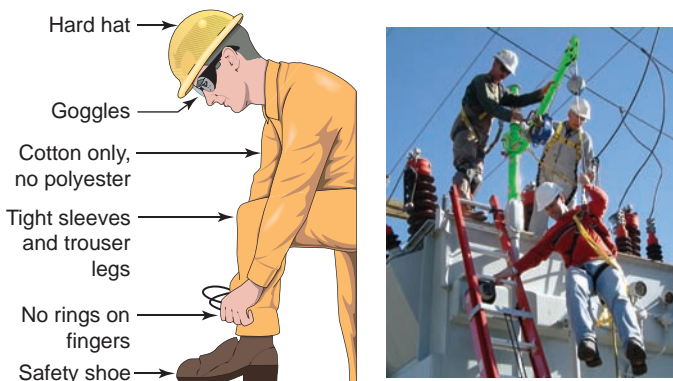
Figure 1-4 Appropriate attire should be worn for each particular job site and work activity.
