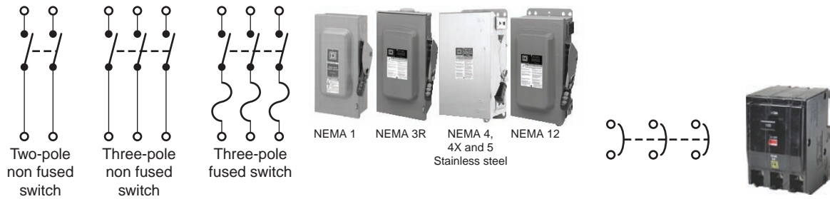
(a) Disconnect switch
