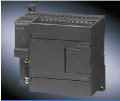
Figure 10-45 Fixed programmable controller. Photos courtesy Siemens, www.siemens.com.
