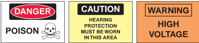
Figure 1-3 Typical safety signs.
