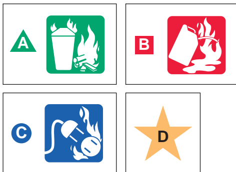
Figure 1-14 Types of fire extinguishers and their applications.
