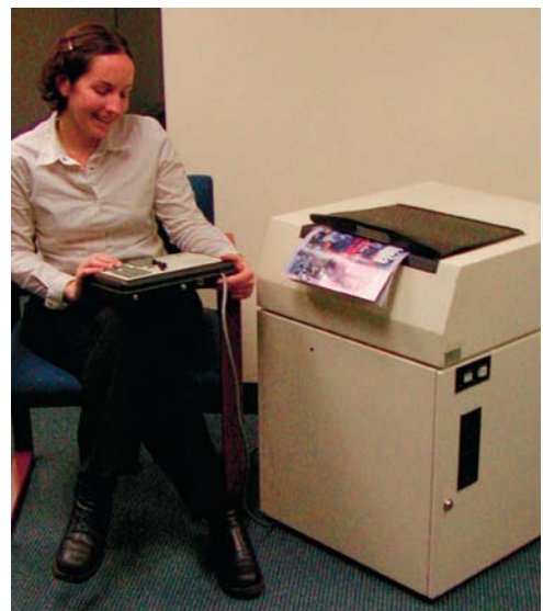
Ray Kuzweil's reading machine for the blind from 1976. This is the first device combining optical scanners, text-to-speech technology and pattern recognition software.
