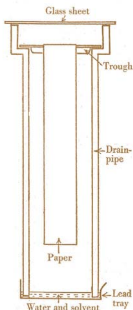
Fig. 3. Elevation of small trough in drain-pipe. 84:3
