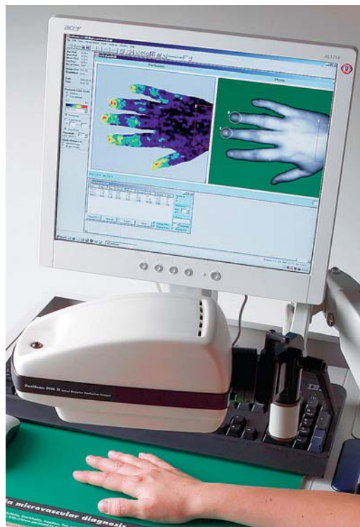
Modern laser Doppler perfusion imaging system showing peripheral circulation in the hand and in the heart during and after coronary by-pass surgery.
