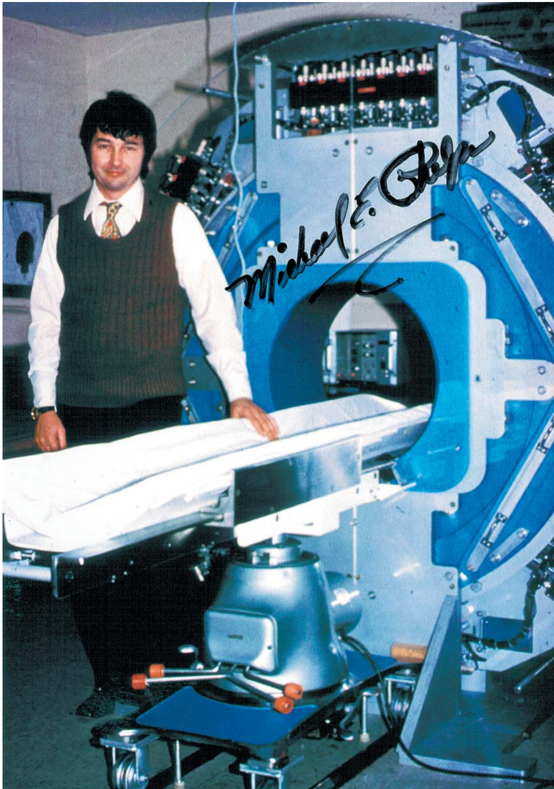
Michael Phelps with the PETT III apparatus, a development of the prototype unit described in the landmark paper from 1975. This device takes the first PET images of blood flow, glucose metabolism and bone scans using Fluorine 18 ( ^{18}\text{F} ) as the radionuclide.
