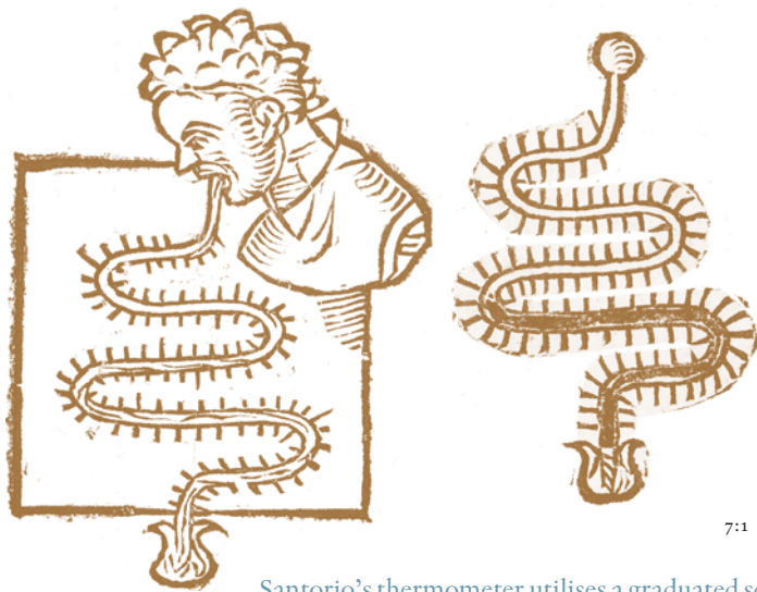
Santorio's thermometer utilises a graduated scale for showing the displacement of a liquid column as the gas volume changes with body temperature.
