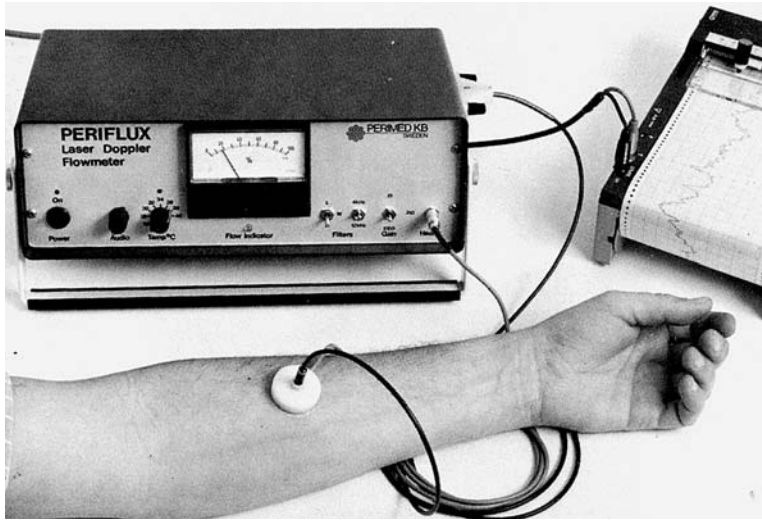
An instrument for microvascular tissue perfusion measurements from the early 1980s.
