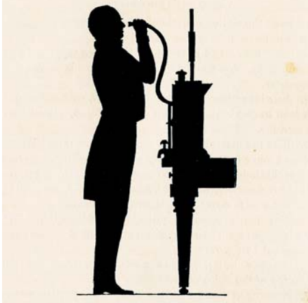
Position of the body in filling the chest before breathing into the Spirometer.
