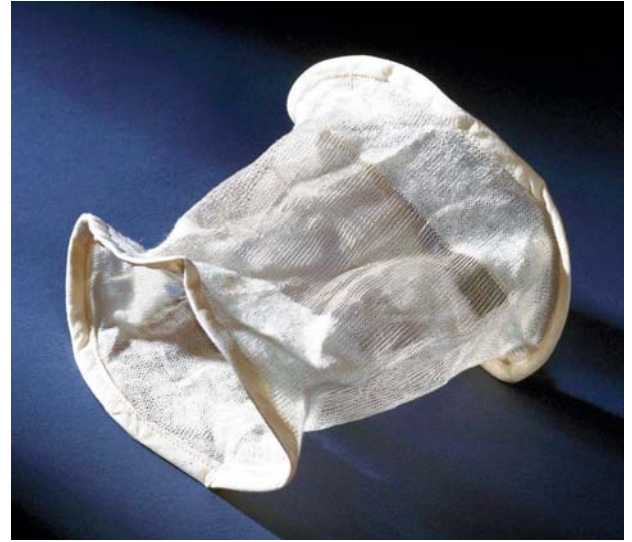
A sample made from the first experimental nylon (polyamide), from 1935.
