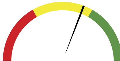
Figure 8.16 An Excel speedometer made of a donut chart.
