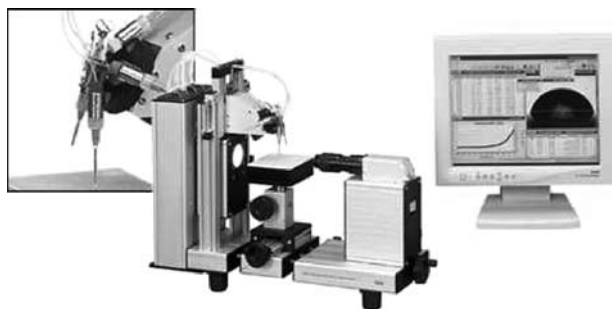
Fig. 6.10 Commercial contact angle device (DSA 10, Fa. Krüss) for measurements with sessile droplets on planar solid surfaces
