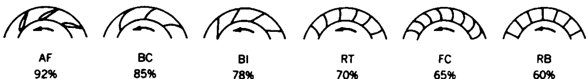
FIGURE 7.1 Six blade shapes commonly used in centrifugal fans. The approximate maximum efficiency attainable for each type is shown. (From Bleier, F. P., Fans, in Handbook of Energy Systems Engineering , New York: Wiley, 1985, used with permission.)
