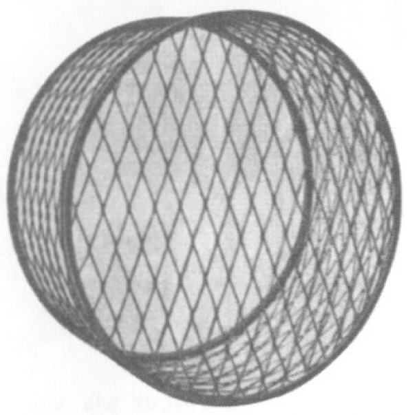
FIGURE 3.8 Fan guard, used for safety and mounted on the inlet side of a propeller fan.
