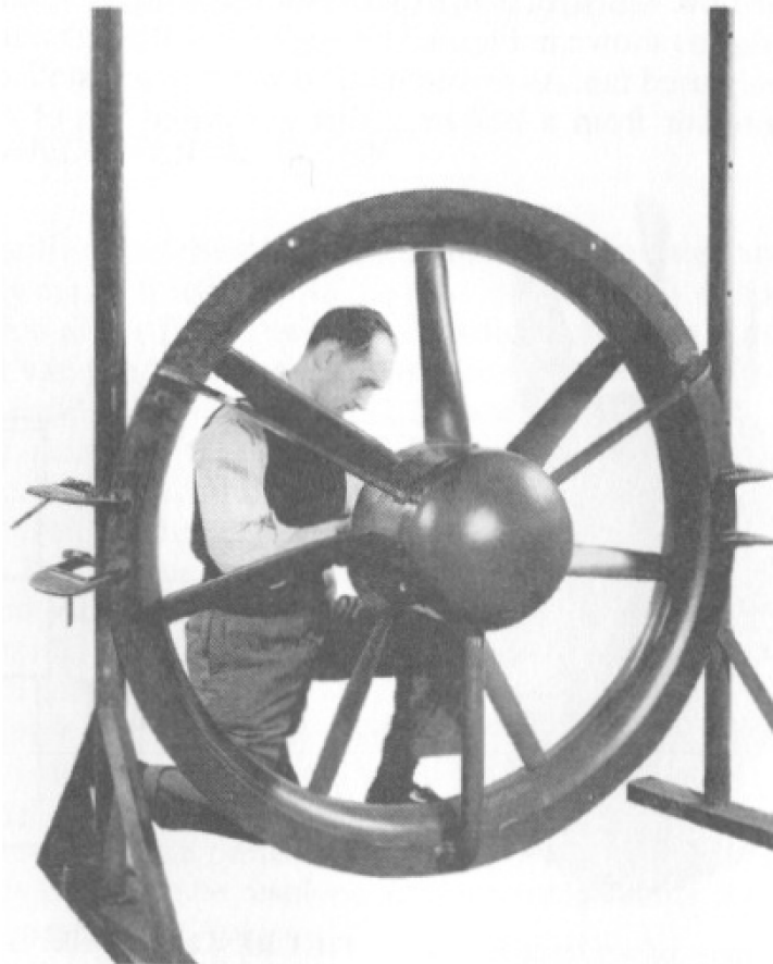
FIGURE 4.4 A 48-in propeller fan with direct drive from a 7\frac{1}{2} -hp, 1150-rpm motor, 28 percent hub-tip ratio, and seven cast-aluminum airfoil blades.
