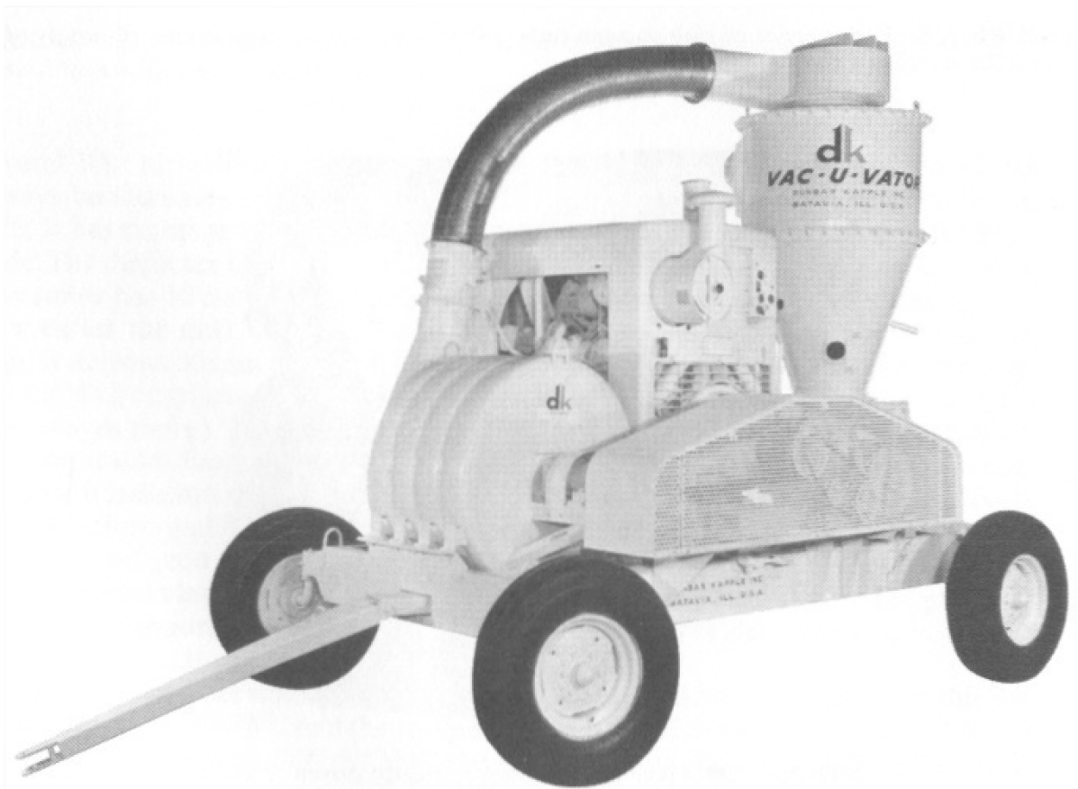
FIGURE 7.41 Four-stage turbo blower, belt drive from 300-hp engine, 26-in wheel diameters, 4800 rpm, for grain conveying. (Courtesy of Christianson Systems, Inc., Blomkest, Minn.)
