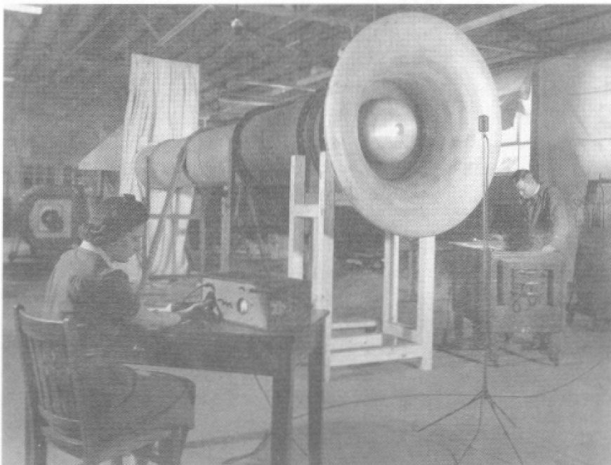
FIGURE 18.16 Microphone and sound level meter measuring the decibels at a certain distance from a vaneaxial fan with an oversize venturi inlet.
