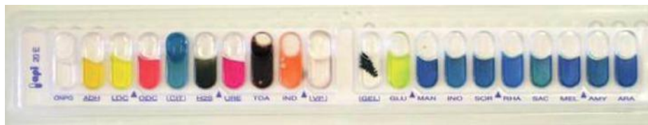
FIGURE 3-2 API™ test demonstrating how bacteria can be differentiated using a series of biochemical tests. Each small compartment contains a dehydrated powder that is inoculated from a bacterial culture. After incubation, the colorimetric changes can be scored numerically to produce a number that matches to a specific bacterial species and genus. (Courtesy of bioMérieux, Inc.)
