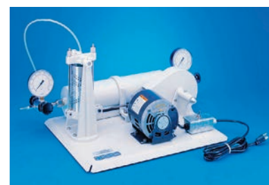
The Parr hydrogenation apparatus shakes the reaction vessel (containing the alkene and the solid catalyst) while a pressurized cylinder supplies hydrogen.
