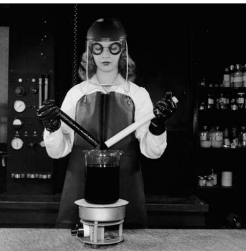
This 1949 DuPont promotional photo shows how a Teflon rod (on our right, in the model's left hand) resists a hot acid solution compared with a rod made from another plastic. In World War II, Teflon was used for insulation in aircraft wiring and for seals in the equipment used to enrich corrosive uranium hexafluoride.
