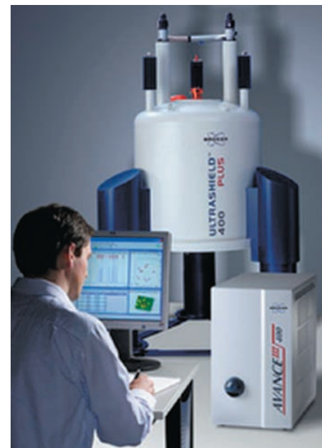
Photo of a 300-MHz NMR spectrometer. The metal container at the back contains the superconducting magnet, cooled by a liquid helium bath. The electronics used to control the spectrometer and to calculate spectra are at right.
