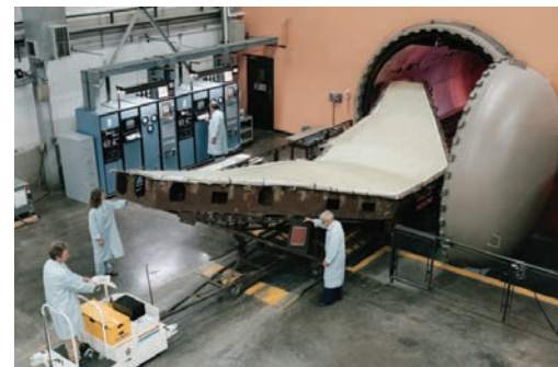
Workers guide the skin for the tail of a Harrier II jet into an autoclave where its layers of epoxy-coated carbon-fiber cloth will be bonded and cured under heat and pressure. The carbon-epoxy composite is used to make aircraft parts that are as strong as steel but as light as aluminum.
