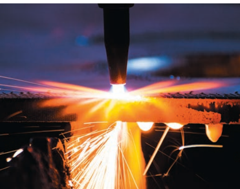
An oxygen–acetylene flame is hot enough to melt steel for welding. A cutting torch uses an extra jet of oxygen to burn away hot steel.
