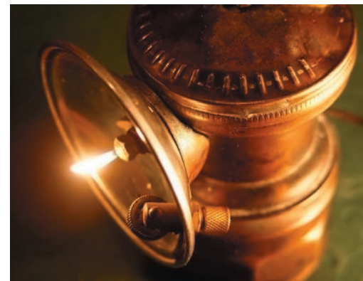
A miner's carbide lamp. Water in the upper chamber slowly drips onto calcium carbide in the lower chamber, generating acetylene.
