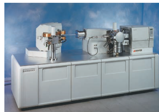
A double-focusing mass spectrometer. This one is combined with a gas chromatograph to use as a GC-MS. The gas chromatograph separates a mixture into its components and injects the purified components into the ion source of the mass spectrometer.
