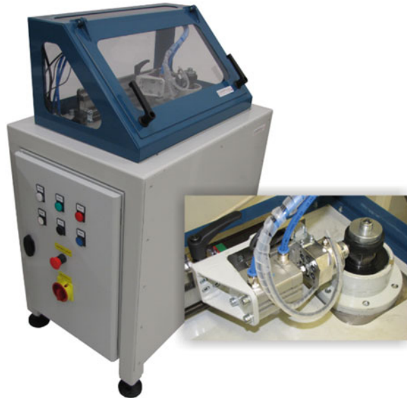
Fig. 27 Photograph of the testing equipment for measurement of dynamic wear
