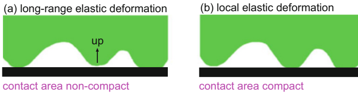
Fig. 2 (a) When a high asperity makes contact with the substrate, the elastic solid in its neighborhood is displaced upwards, making it less likely for nearby smaller asperities to make contact with the substrate. This results in a more open contact morphology than expected if the long-range elastic coupling is neglected (see (b)), as is the case in the GW (and most other) asperity contact mechanics models
