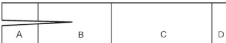
Fig. 3 Characteristic regions (A–D) of a loaded single-edge notched PS specimen [3]
