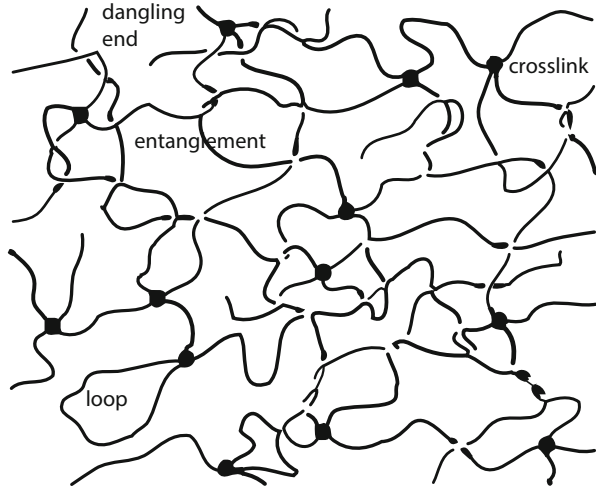
Fig. 5 Different structural elements in a network. Entanglements and knots contribute to the elasticity, dangling ends and self-crosslinked loops do not
