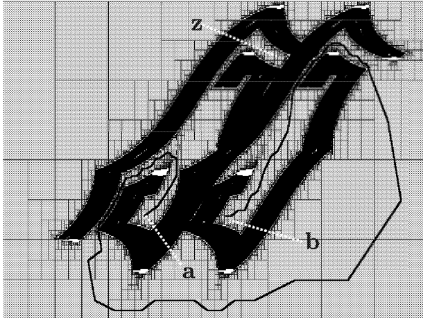
Fig. 8.12. Paving and path generated by FEASIBLEPATH1; the frame corresponds to the search box [p_0] = [-28, 57] \times [-1.4, 2.7] ; z corresponds to a dead-end
