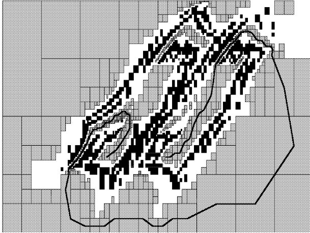
Fig. 8.14. Paving and path generated by FEASIBLEPATH2. The frame corresponds to the search box [\mathbf{p}_0] = [-28, 57] \times [-1.4, 2.7]
